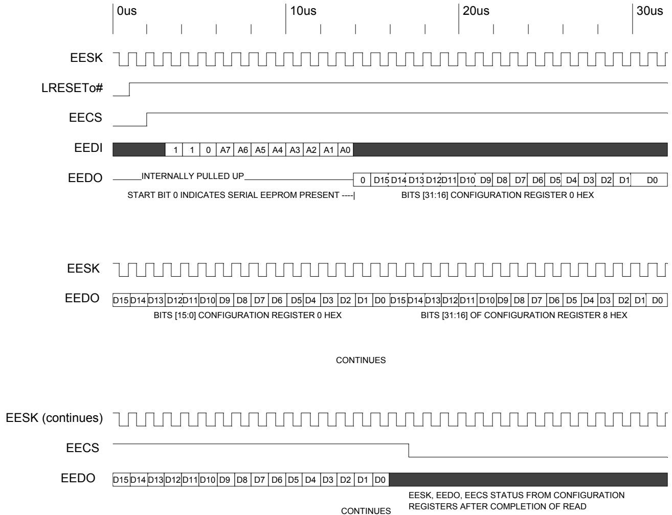
Timing Diagram 3-1. Initialization from Serial EEPROM (2K or 4K Bit)
