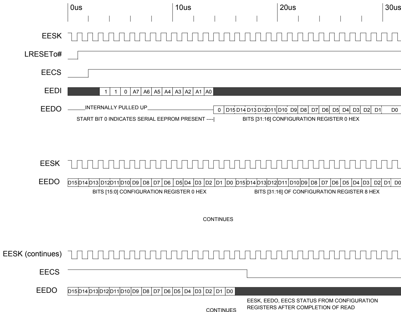
Timing Diagram 4-2. Initialization from Serial EEPROM (2K or 4K Bit)
