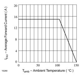
Figure 1. Max. Average Forward Current vs.
