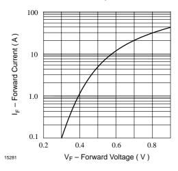
Figure 2. Typ. Forward Current vs. Forward Voltage
