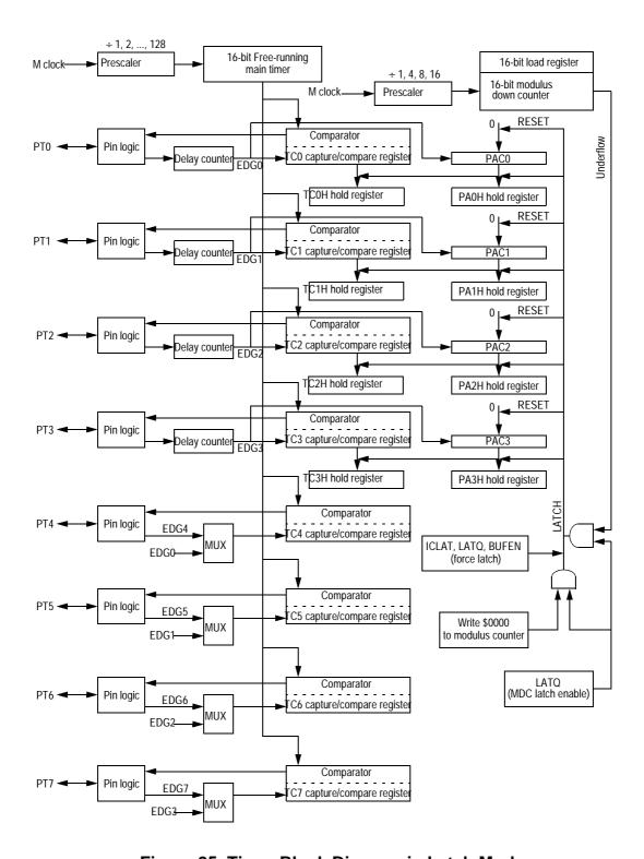
Figure 25 Timer Block Diagram in Latch Mode
