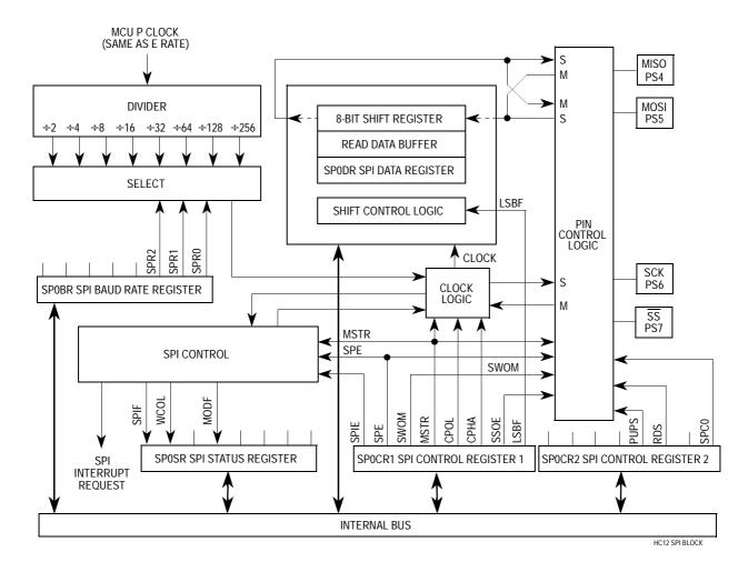
Figure 33 Serial Peripheral Interface Block Diagram
