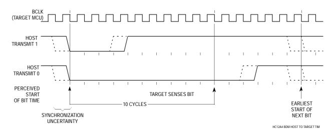
Figure 59 BDM Host to Target Serial Bit Timing
