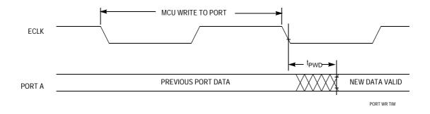
Figure 68 Port Write Timing Diagram
