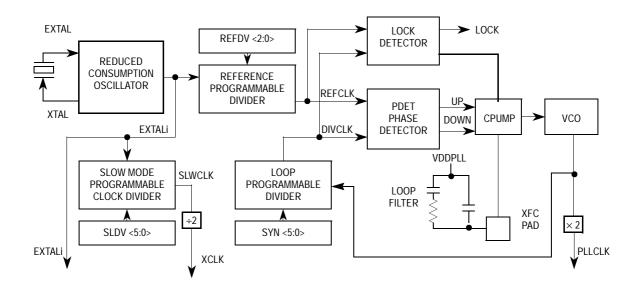
Figure 14 PLL Functional Diagram
