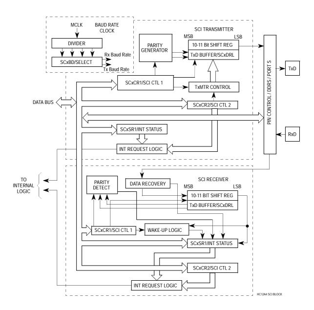
Figure 32 Serial Communications Interface Block Diagram
