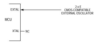
**Figure 9 External Oscillator Connections**
