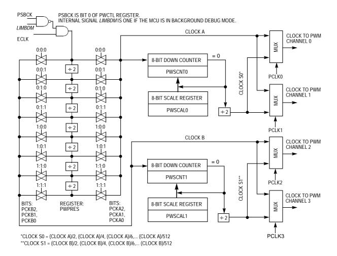
Figure 24 PWM Clock Sources
