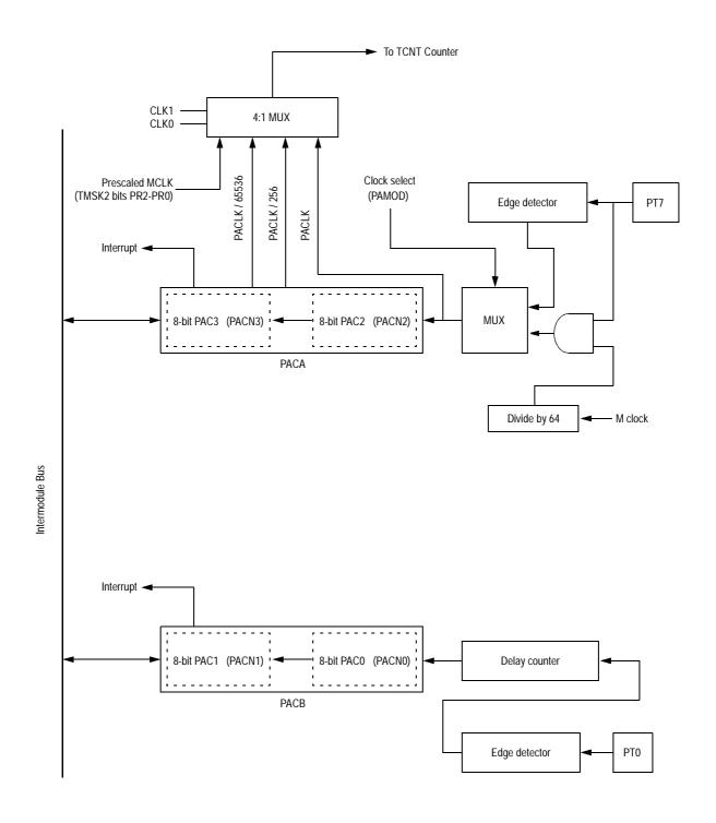
Figure 28 16-Bit Pulse Accumulators Block Diagram
