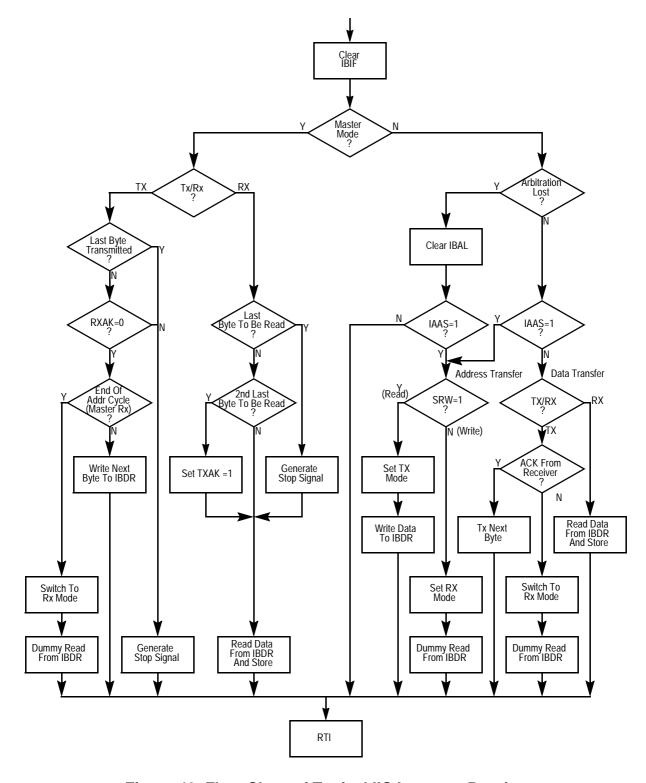
Figure 40 Flow-Chart of Typical IIC Interrupt Routine
