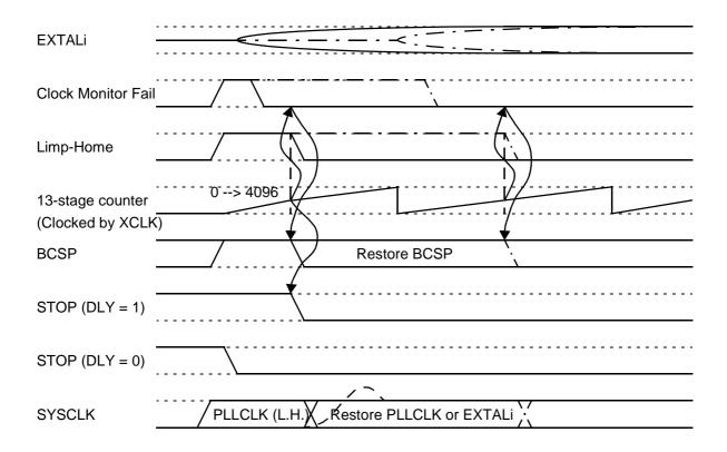
Figure 17 STOP Exit and Fast STOP Recovery
