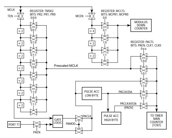
Figure 20 Clock Chain for ECT
