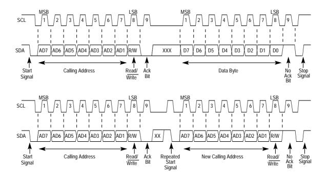
Figure 38 IIC Transmission Signals
