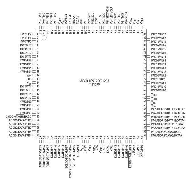
Note: TEST = On early production devices this pin is used for factory test purposes. It is recommended that this pin is not connected within the application, but it may be connected to VSS or 5.5V max without issue.
