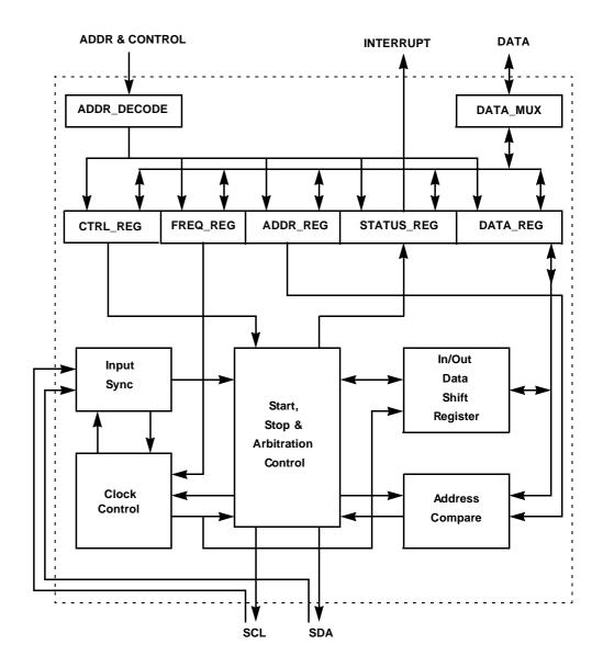
Figure 37 IIC Block Diagram
