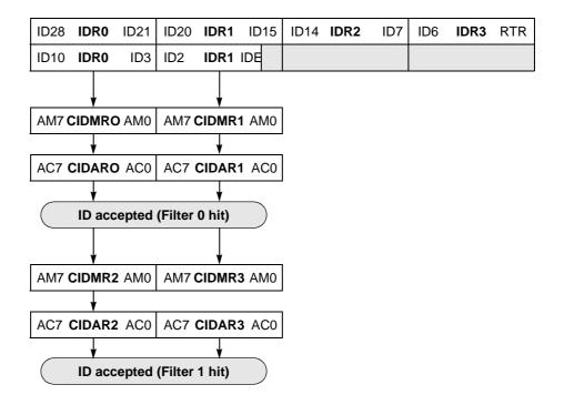
Figure 44 16-bit Maskable Acceptance Filters
