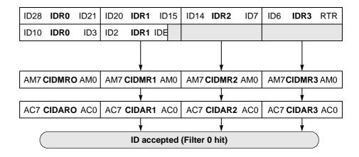
Figure 43 32-bit Maskable Identifier Acceptance Filters
