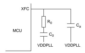
Figure 7 PLL Loop Filter Connections
