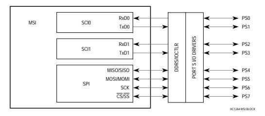
Figure 31 Multiple Serial Interface Block Diagram
