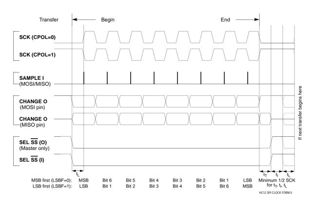
Figure 34 SPI Clock Format 0 (CPHA = 0)
