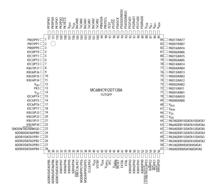
Note: TEST = On early production devices this pin is used for factory test purposes. It is recommended that this pin is not connected within the application, but it may be connected to VSS or 5.5V max without issue.
