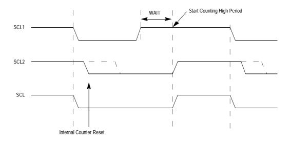
Figure 39 IIC Clock Synchronization
