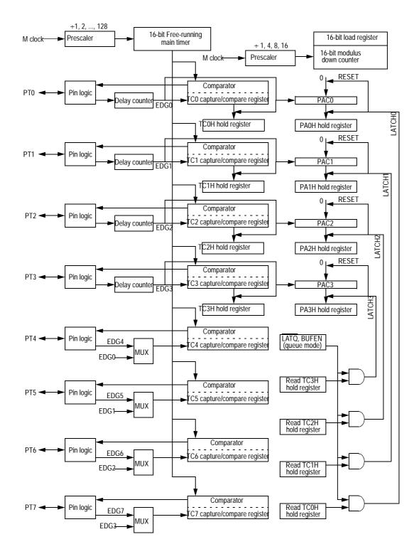
Figure 26 Timer Block Diagram in Queue Mode
