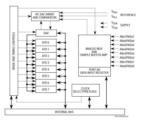
Figure 58 Analog-to-Digital Converter Block Diagram
