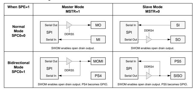
Figure 36 Normal Mode and Bidirectional Mode
