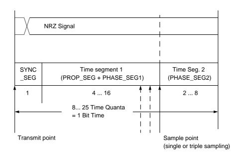
Figure 48 Segments within the Bit Time
