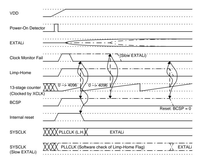
Figure 16 No Clock at Power-On Reset
