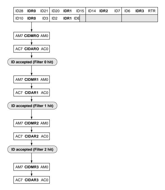
Figure 45 8-bit Maskable Acceptance Filters
