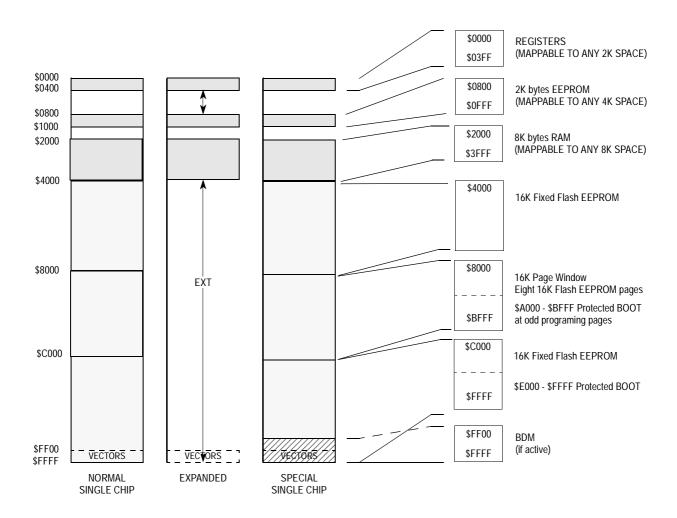
Figure 10 MC68HC912DT128A Memory Map after reset
