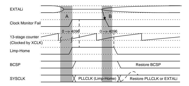
Figure 15 Clock Loss during Normal Operation
