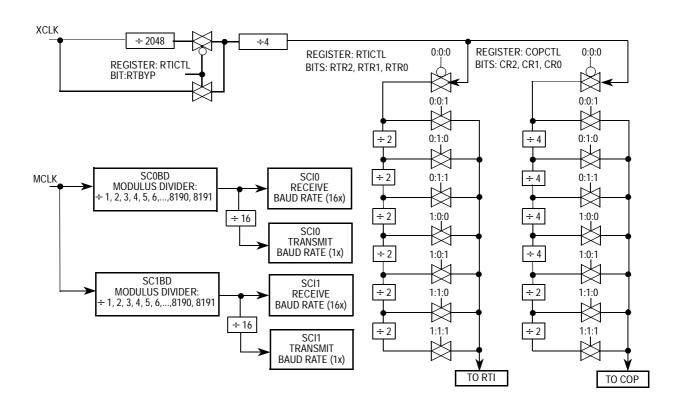
Figure 19 Clock Chain for SCI0, SCI1, RTI, COP
