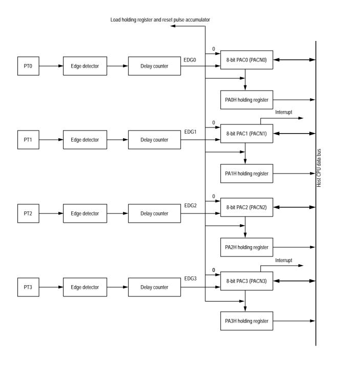
Figure 27 8-Bit Pulse Accumulators Block Diagram
