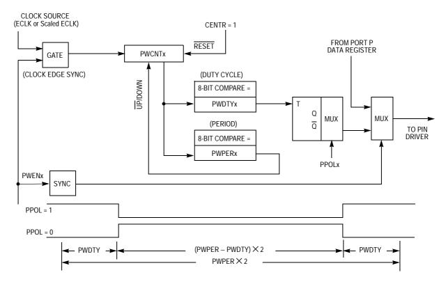
Figure 23 Block Diagram of PWM Center-Aligned Output Channel
