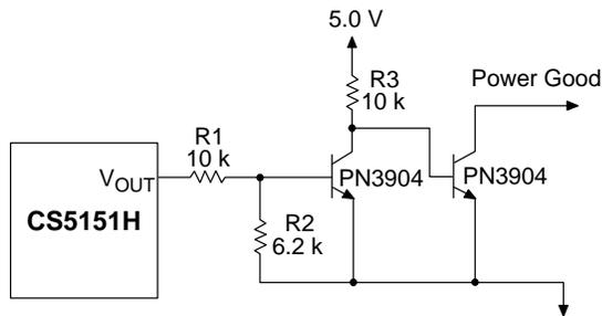
**Figure 15. Implementing Power Good with the CS5151H**
