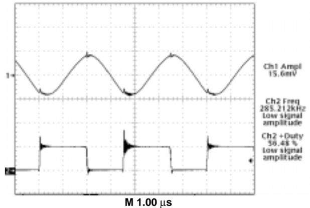
Trace 1– Regulator Output Voltage (10 mV/div.)
