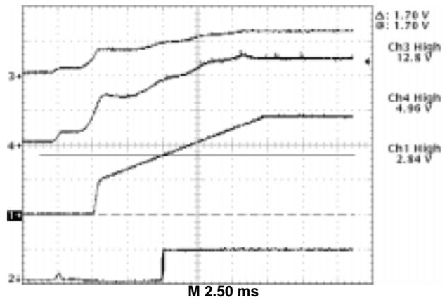
Trace 3 – 12 V Input ( $V_{CC1}$ ) and ( $V_{CC2}$ ) (10 V/div.)
