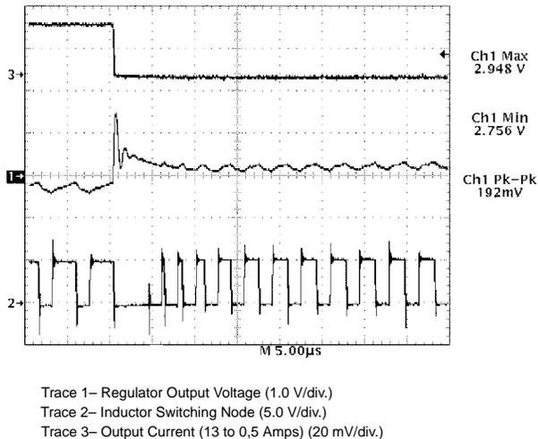
**Figure 11. CS5151H Demonstration Board Response to 13 A Load Turn Off (Output Set for 2.8 V). V<sup>2</sup> Control Topology Immediately Connects Inductor to Ground, Providing 0% Duty Cycle. Regulation is Achieved in Less Than 10 µs**
