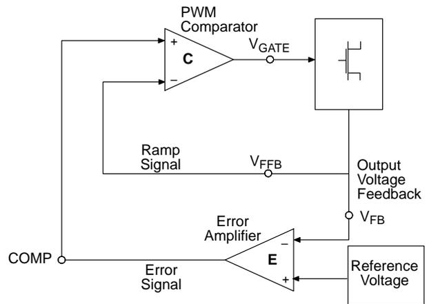
Figure 3. V<sup>2</sup> Control Diagram
