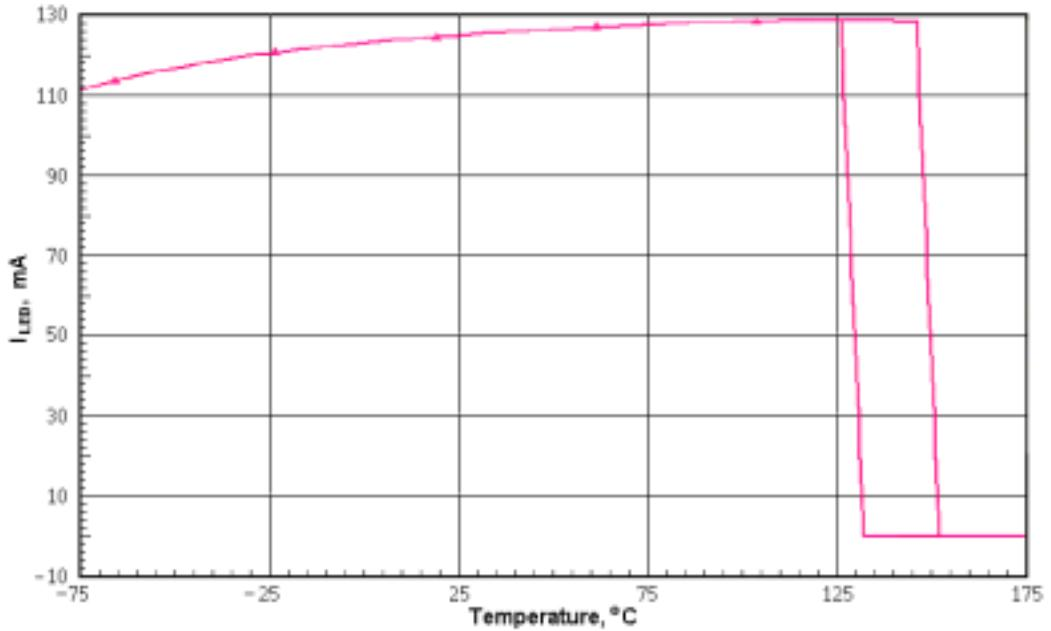
Figure 6 – LED Current versus Temperature with Thermal Shutdown
