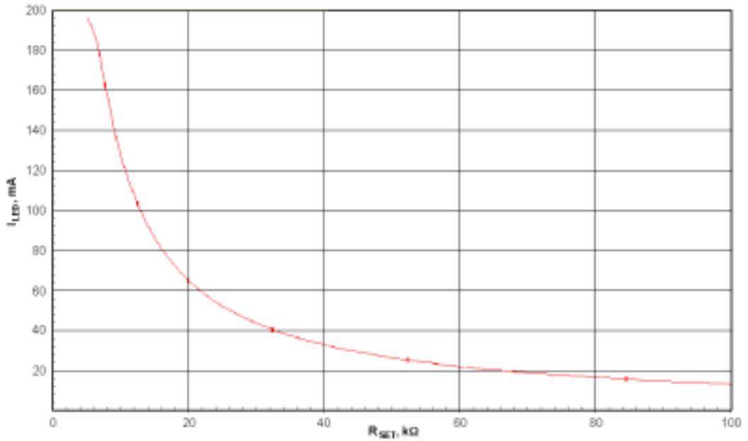
Figure 5 – LED Current versus  $R_{SET}$  Value
