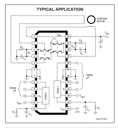
sequence. This is accomplished by digitally selecting 100% drive current when only one phase is ON and 67% drive current when two phases are ON. Logic highs on both  $I_0$  and  $I_1$  turn OFF all drivers to allow rapid current decay when switching phases. This helps to ensure proper motor operation at high step rates.
