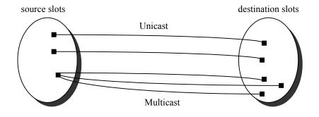
tbsMapSlot establishes the mapping between the source space-time slot and the destination space-time slot(s). tbsRmSlot disconnects the established connection between the given source and destination slots. tbsClrSlot clears all connections for the given source slot.
