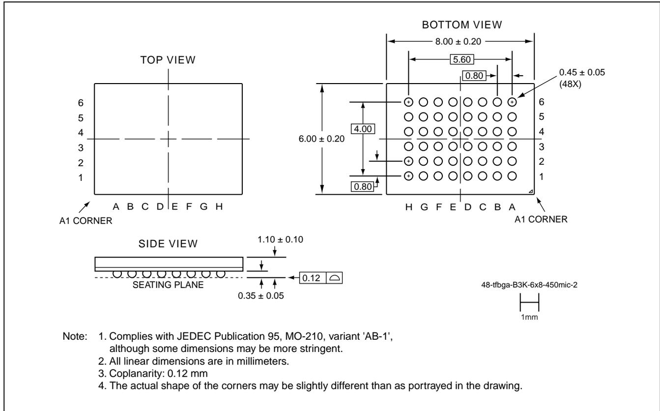
**48-BALL THIN-PROFILE, FINE-PITCH BALL GRID ARRAY (TFBGA) 6MM X 8MM**
