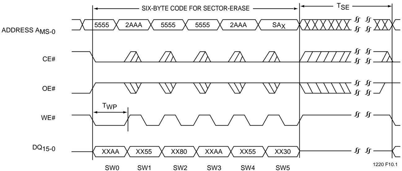
**Note:** This device also supports CE# controlled Sector-Erase operation. The WE# and CE# signals are interchangeable as long as minimum timings are met. (See Table 13)
