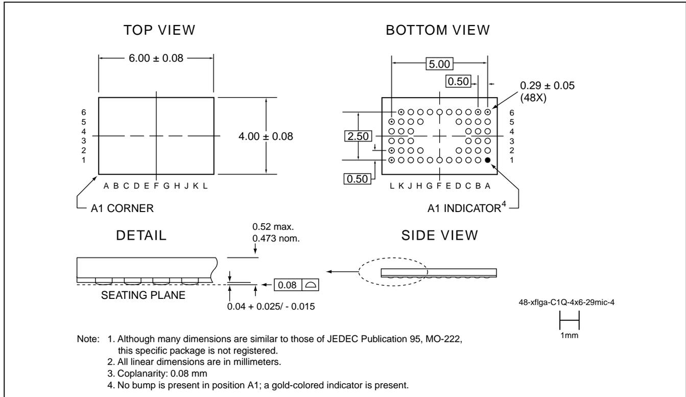
**48-BUMP ULTRA-ULTRA-THIN-PROFILE, FINE-PITCH LAND GRID ARRAY (XFLGA) 4MM X 6MM**
