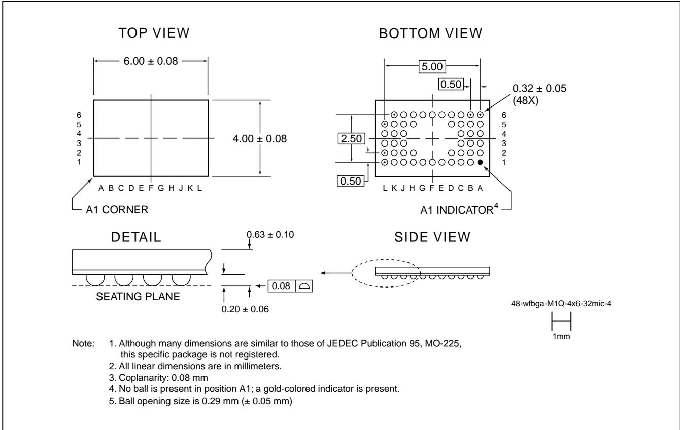
**48-BALL ULTRA-THIN-PROFILE, FINE-PITCH BALL GRID ARRAY (WFBGA) 4MM X 6MM**
