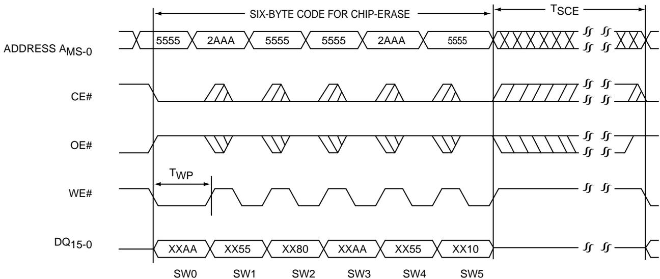
**Note:** This device also supports CE# controlled Chip-Erase operation. The WE# and CE# signals are interchangeable as long as minimum timings are met. (See Table 13)
