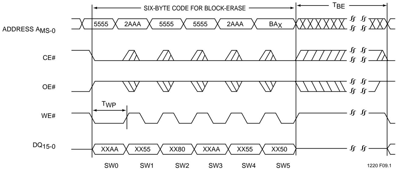
**Note:** This device also supports CE# controlled Block-Erase operation. The WE# and CE# signals are interchangeable as long as minimum timings are met. (See Table 13)
