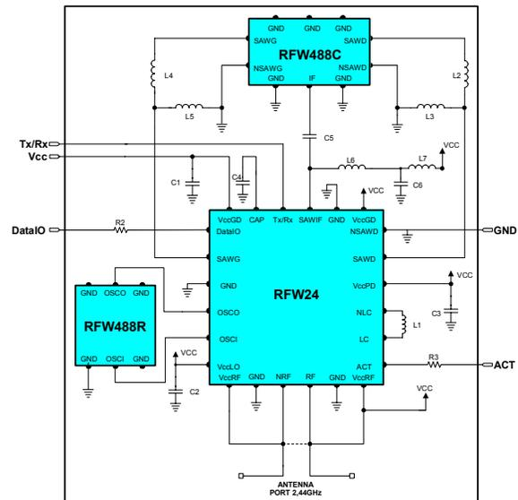
Figure 2: Transceiver Implementation - Using RFW102 Chipset
