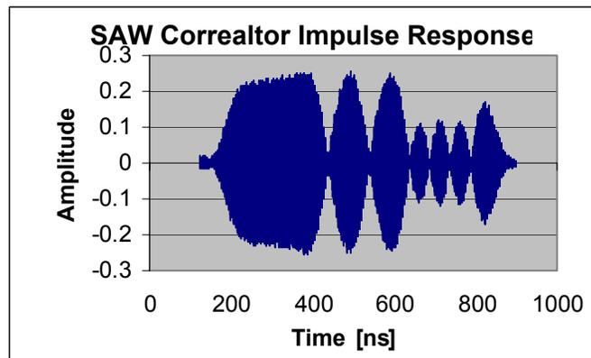
Figure 5: Pulse Response of the Correlator - Measured
