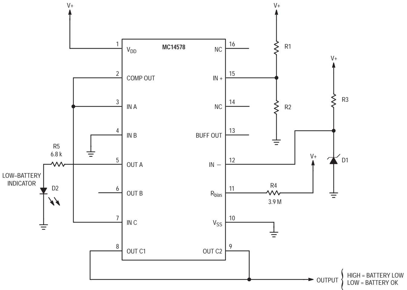
NOTE: IN + and IN - have very high input impedance. Interconnect to these pins should be as short as possible.
