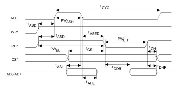
Figure 23-2 **INTEL BUS WRITE TIMING (BTS=0 / MUX=1)**
