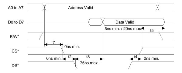
Figure 23-7 MOTOROLA BUS WRITE TIMING (BTS=1 / MUX=0)
