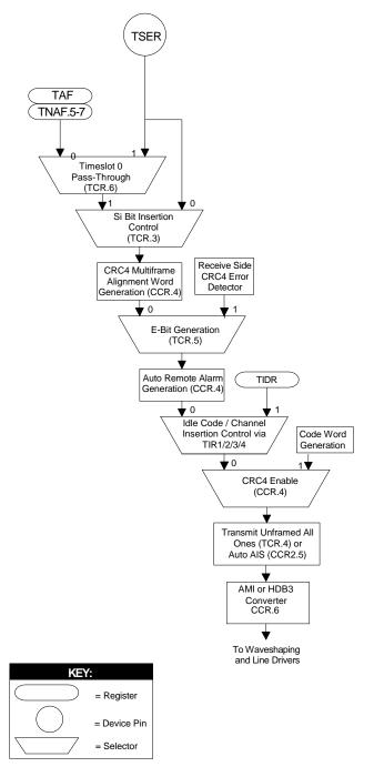
Figure 21-9 **DS21Q50 TRANSMIT DATA FLOW**
