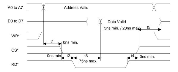
Figure 23-5 INTEL BUS WRITE TIMING (BTS=0 / MUX=0)
