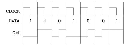
Transmit and Receive CMI is enabled via OUTAC.7. When this register bit is set, the TTIP pin will output CMI coded data at normal TTL type levels. This signal can be used to directly drive an optical interface. When CMI is enabled, the user may also use HDB3 coding.
