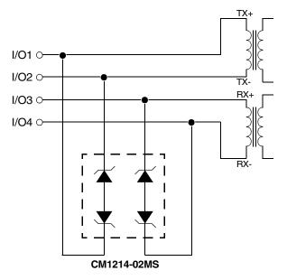
Figure 5. Typical Application - Ethernet Protection, CM1214-02MS in 8-lead MSOP
