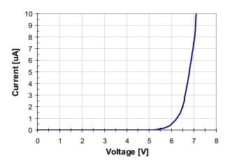
Figure 2. CM1214 VI Characteristics, Low Current
