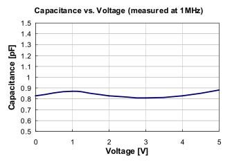
Figure 1. CM1214 Capacitance VS. Voltage
