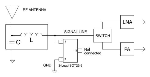
Figure 4. Typical Application - RF Switch and Amplifier Protection, CM1214-01ST in 3-lead SOT23
