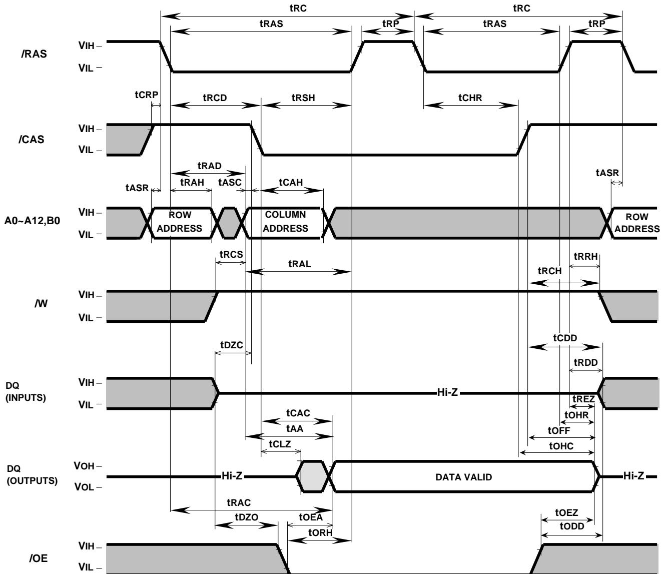
Note 31: Early write, delayed write, read write or read modify write cycle is applicable instead of read cycle.
