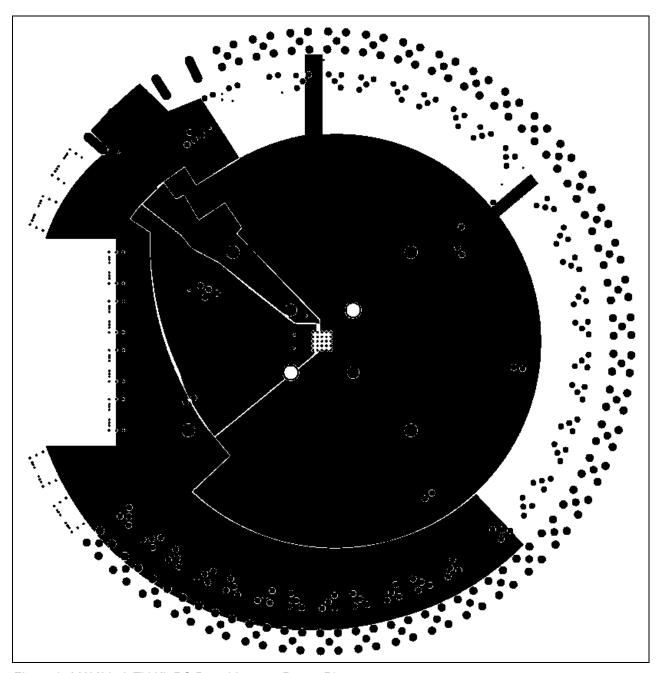
Figure 9. MAX3952 EV Kit PC Board Layout-Power Plane
