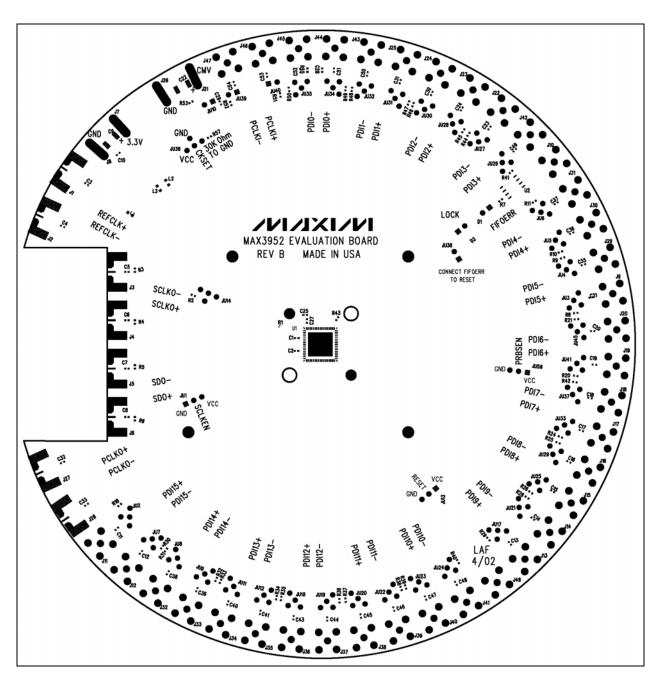
Figure 4. MAX3952 EV Kit Placement Guide-Component Side
