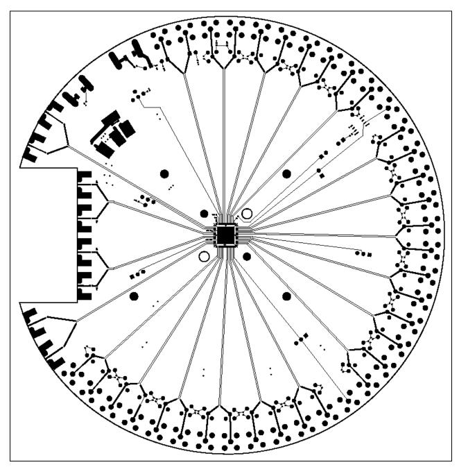
Figure 7. MAX3952 EV Kit PC Board Layout–Component Side
