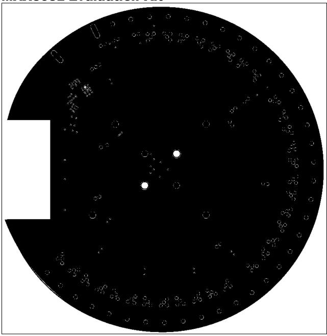
Figure 8. MAX3952 EV Kit PC Board Layout-Ground Plane
