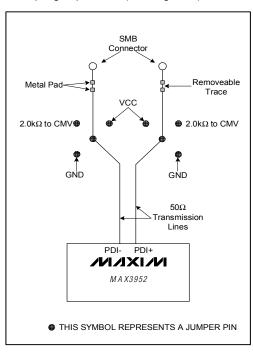
Figure 1. Detail of PDI± Inputs
