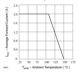
Figure 1. Max. Average Forward Current vs.
