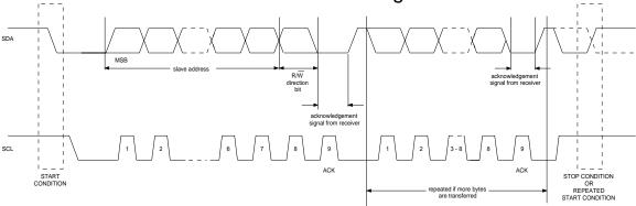
Figures 5 and 6 detail how data transfer is accomplished on the 2-wire bus. Depending upon the state of the  $R/\overline{W}$  bit, two types of data transfer are possible:
