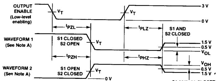
For the 'LS793, the latch control "G" should be low while testing the enable and disable times, so that the output (Q) does not change. ( $V_T = 1.3V$ ).
