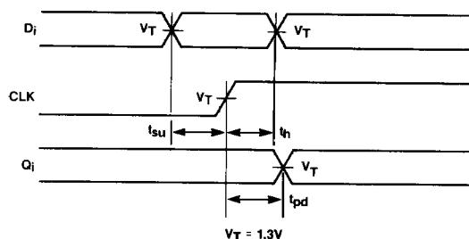
The case when gate is HIGH and data flows through the part is specified as Data to Output delay in the Switching Characteristics table. ( $V_T = 1.3V$ ).
