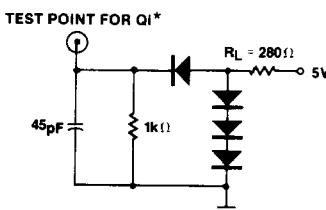
\* The "TEST POINT" is driven by the output under test, and observed by instrumentation.
