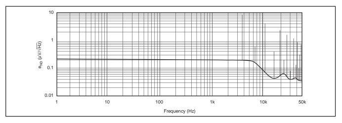
Figure 10. V<sub>OUT</sub> Noise Spectrum for Coarse Offset Adjust = -56mV, Gain = 1152, CLK\_CFG = '00' (default).
