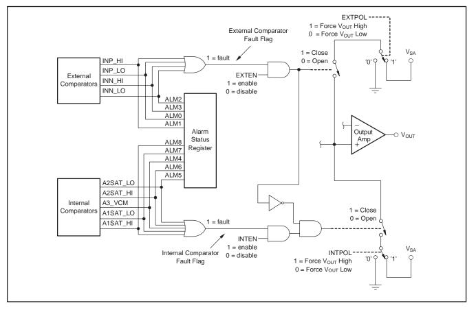
Figure 20. Fault Monitor Comparator Logic
