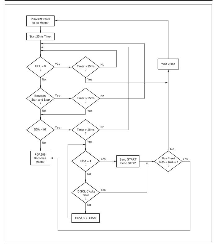
Figure 56. Two-Wire Bus Master Algorithm
