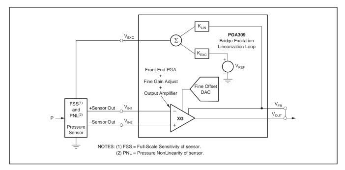
Figure 25. Bridge Excitation Linearization Loop
