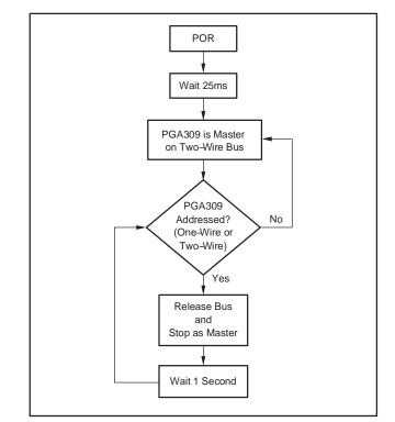
Figure 55. Two-Wire Bus Relinquish by PGA309 in Master Mode
