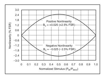
Figure 28. Parabolic Bridge Nonlinearity vs Pressure
