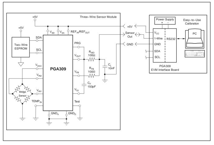
Figure 57. One-Wire Operation with PRG Tied to  $\mathsf{V}_{\text{OUT}}$
