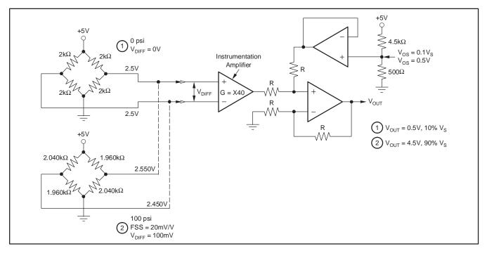
Figure 66. Ratiometric Configuration, 5V
