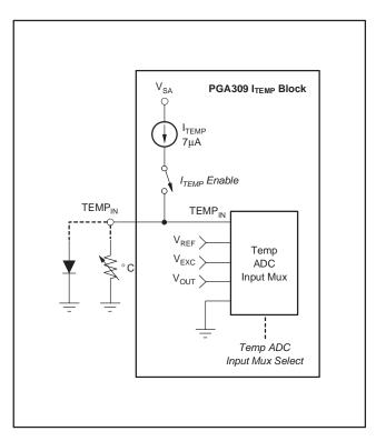
Figure 32. ITEMP for External Temperature Measurement
