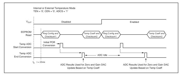
Figure 34. Temp ADC Single Start-Convert Control
