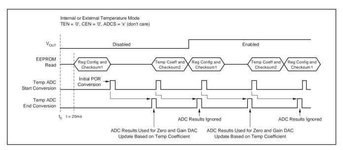
Figure 33. Temp ADC Continuous Start-Convert Control
