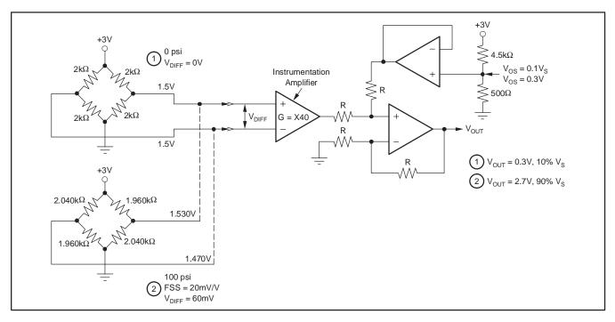
Figure 67. Ratiometric Configuration, 3V
