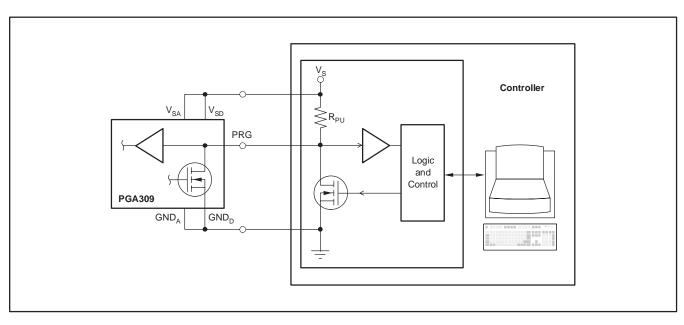
Figure 47. Typical PGA309 PRG To Controller Connection
