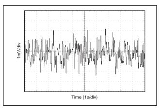
Figure 9. 0.1Hz to 10Hz V<sub>OUT</sub> Peak-to-Peak Noise for Coarse Offset Adjust = -59mV, Gain = 1152, V<sub>IN</sub> = +61mV.
