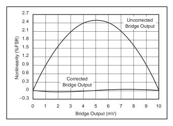
Figure 24. Bridge Pressure Nonlinearity Correction
