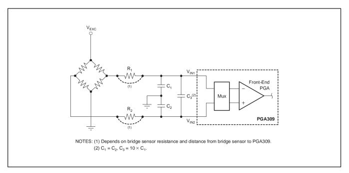
Figure 40. Input Filtering
