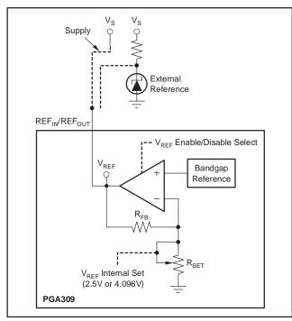
Figure 17. PGA309 Reference Circuit
