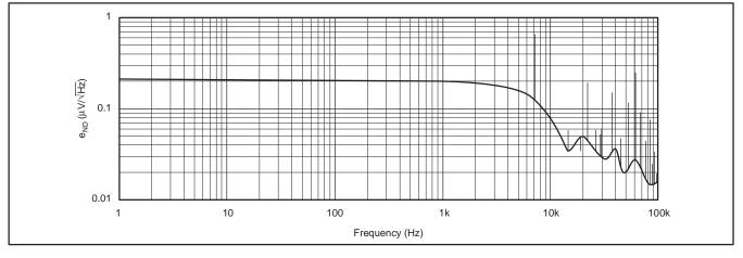
Figure 6. V<sub>OUT</sub> Noise Power Spectrum for Coarse Offset Adjust = 0mV, Gain = 1152, CLK\_CFG = '00' (default).
