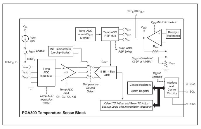
Figure 30. Temperature Sense Block
