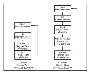
Figure 49. One-Wire Access to PGA309 Registers
