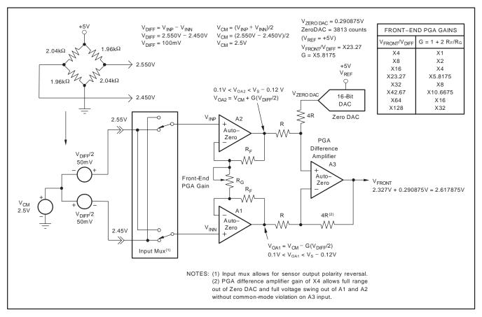
Figure 3. Front-End PGA Gain
