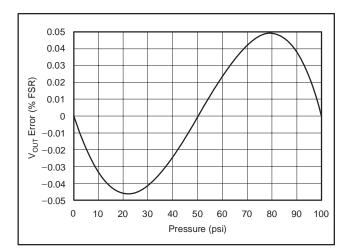
Figure 29. Parabolic Bridge Corrected Nonlinearity vs Pressure
