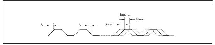
Figure 51. One-Wire Timing Diagram
