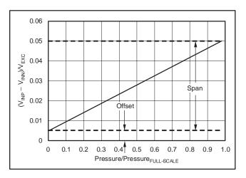
Figure 60. Example of Span and Offset
