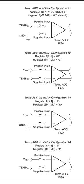
Figure 31. Temp ADC Input Mux Options
