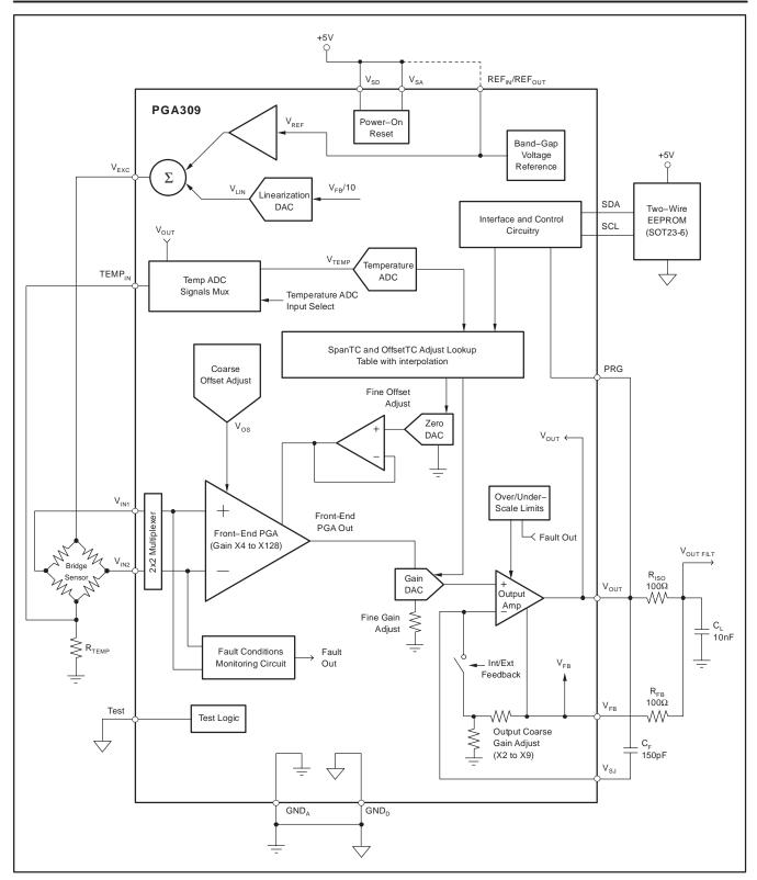
Figure 1. Simplified Diagram of the PGA309
