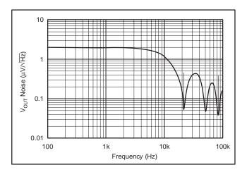
Figure 16.  $V_{OUT}$  Noise Spectrum for Coarse Offset Adjust = -56mV, Gain = 1152,  $V_{IN}$  = +57mV, CLK\_CFG = '11'.
