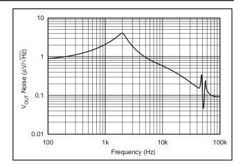
Figure 15. V<sub>OUT</sub> Noise Spectrum for Coarse Offset Adjust = -56mV, Gain = 1152, V<sub>IN</sub> = +57mV, CLK\_CFG = '10'.
