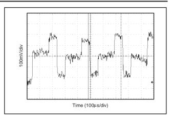
Figure 8. V<sub>OUT</sub> Clock Feedthrough Glitch, Coarse Offset Adjust = 59mV, Gain = 1152, CLK\_CFG = '00' (default). V<sub>OUT</sub> Glitch (RTI) =  $347\mu$ V<sub>PP</sub>.
