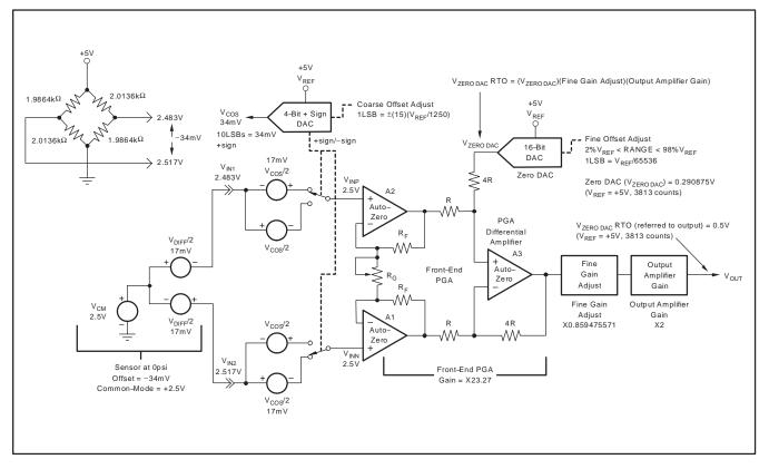
Figure 5. Coarse and Fine Offset Adjust
