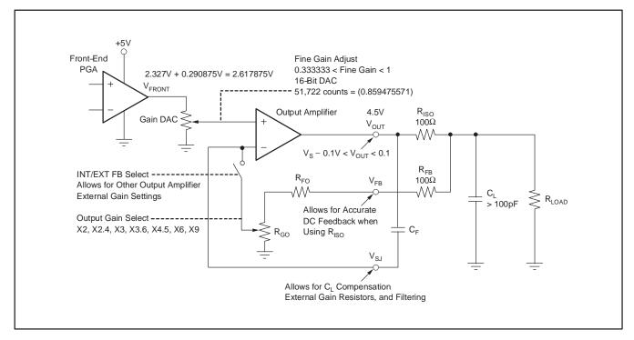
Figure 4. Fine Gain Adjust of the PGA309
