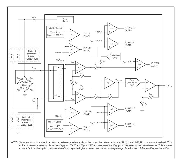
Figure 19. PGA309 Fault Monitor Circuitry
