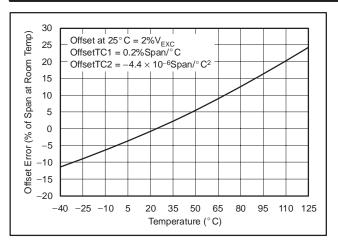
Figure 63. Effect of Nonlinearity on Bridge Sensor Offset Over Temperature
