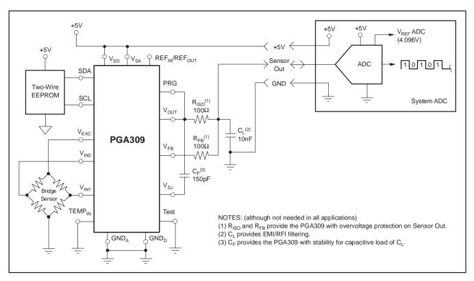
Figure 22. Absolute Scale System—PGA309 Connected to a System ADC
