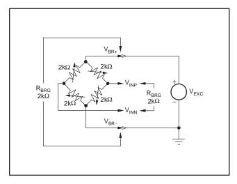
Figure 59. Typical Bridge Sensor
