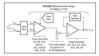
Figure 2. Gain Blocks of the PGA309
