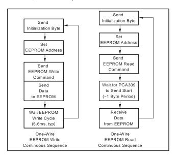
Figure 50. One-Wire Access to External EEPROM
