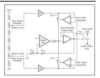
Figure 21. Over-Scale and Under-Scale Limit Circuit
