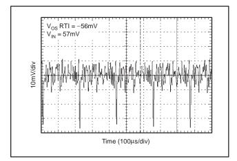
Figure 14. 0.1Hz to 10Hz V<sub>OUT</sub> Peak-to-Peak Noise for Coarse Offset Adjust = -56mV, Gain = 1152, V<sub>IN</sub> = +57mV, CLK\_CFG = '11', V<sub>NPP</sub> (RTI) =  $42\mu V_{PP}$ .
