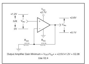
Figure 39. Output Amplifier Minimum Gain at Low Supply
