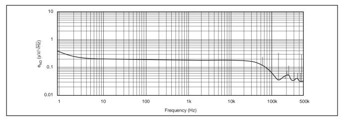
Figure 12. V<sub>OUT</sub> Noise Spectrum for Coarse Offset Adjust = -56mV, Gain = 1152, V<sub>IN</sub> = +57mV, CLK\_CFG = '01'.
