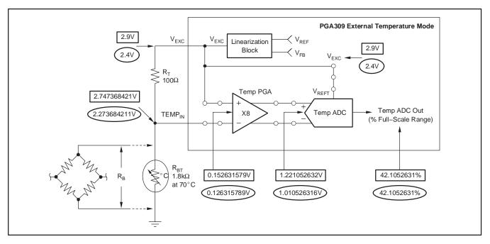
Figure 35. External Temperature Sensing of Bridge Sensor with Top-Side Series Resistor
