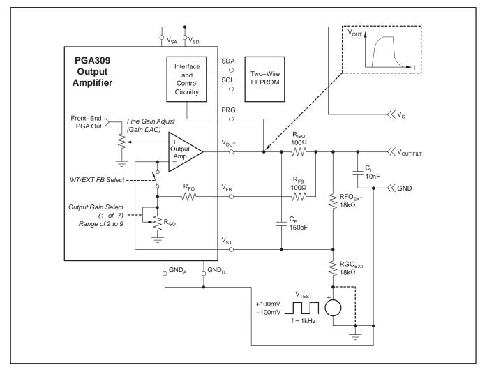
Figure 38. Output Amplifier Using External Feedback Resistors RFO<sub>EXT</sub> and RGO<sub>EXT</sub>
