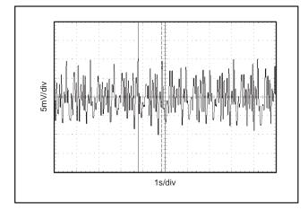
Figure 13. 0.1Hz to 10Hz V<sub>OUT</sub> Peak-to-Peak Noise for Coarse Offset Adjust = -56mV, Gain = 1152, V<sub>IN</sub> = +57mV, CLK\_CFG = '10', V<sub>NPP</sub> (RTI) =  $18.4\mu V_{PP}$ .
