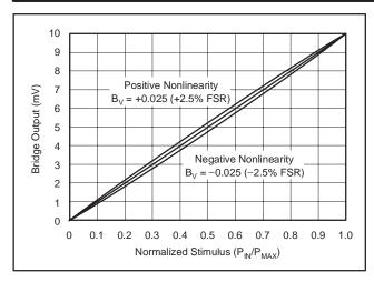
Figure 27. Parabolic Bridge Output vs Pressure
