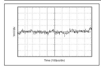
Figure 7. V<sub>OUT</sub> Clock Feedthrough for Coarse Offset Adjust = 0mV, Gain = 1152, CLK\_CFG = '00' (default).
