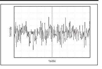
Figure 11. 0.1Hz to 10Hz V<sub>OUT</sub> Peak-to-Peak Noise for Coarse Offset Adjust = -56mV, Gain = 1152, V<sub>IN</sub> = +57mV, CLK\_CFG = '01', V<sub>NPP</sub> (RTI) =  $4.44\mu$ V<sub>PP</sub>.
