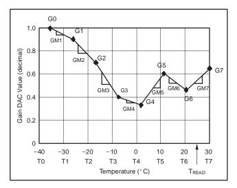
Figure 18. Gain DAC Temperature Coefficients— Definition Example
