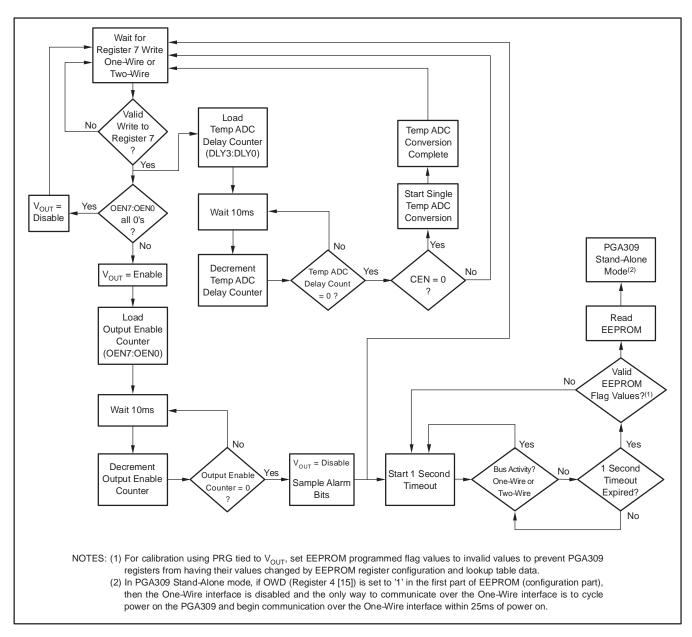
Figure 58. Output Enable/Disable State Machine
