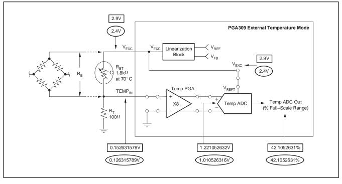
Figure 36. External Temperature Sensing of Bridge Sensor with Bottom-Side Series Resistor
