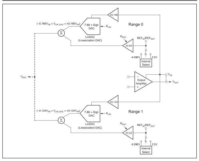
Figure 26. Linearization Circuitry
