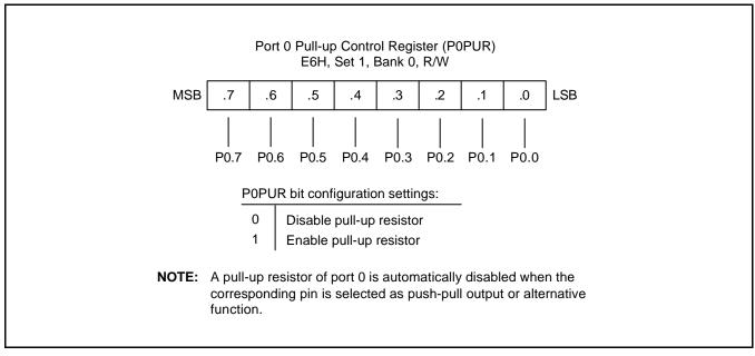
Figure 9-4. Port 0 Pull-up Control Register (P0PUR)
