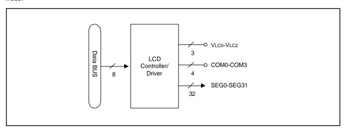
Figure 13-1. LCD Function Diagram
