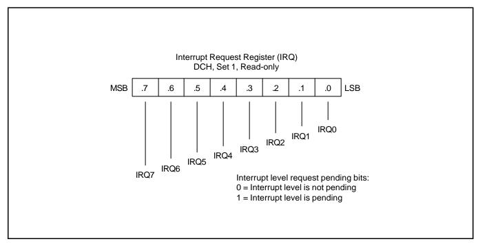
Figure 5-9. Interrupt Request Register (IRQ)
