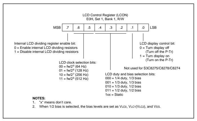
Figure 13-4. LCD Control Register (LCON)
