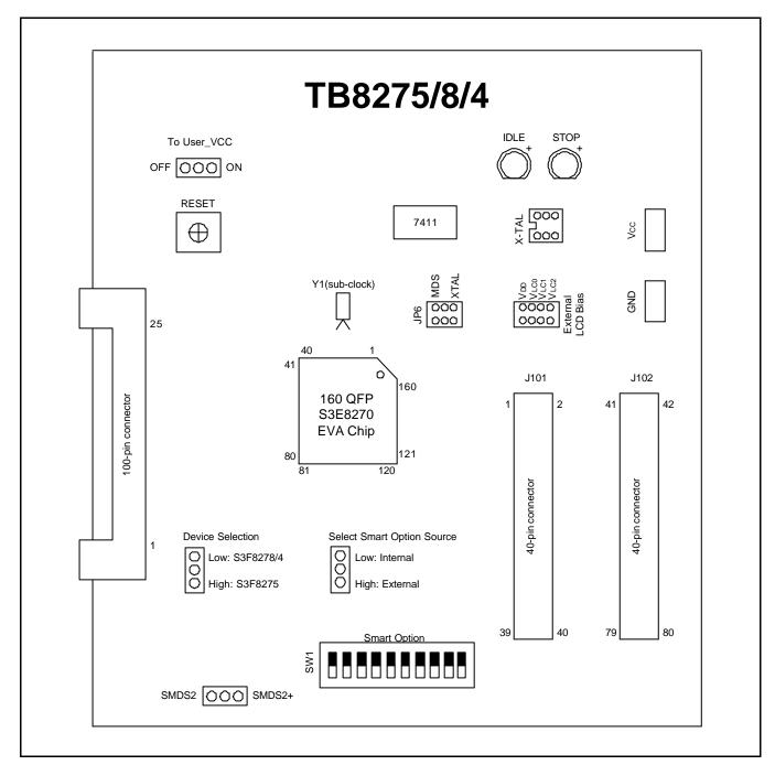
Figure 20-2. TB8275/8/4 Target Board Configuration
