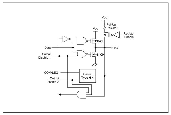
Figure 1-9. Pin Circuit Type H-9 (P4, P5, P6)
