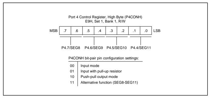
Figure 9-19. Port 4 High-Byte Control Register (P4CONH)
