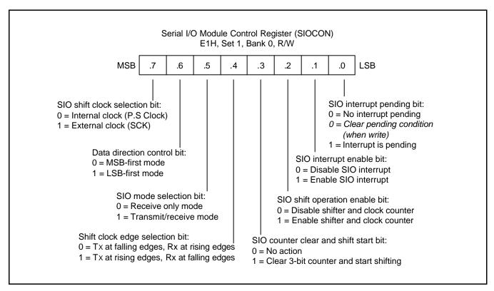
Figure 14-1. Serial I/O Module Control Register (SIOCON)
