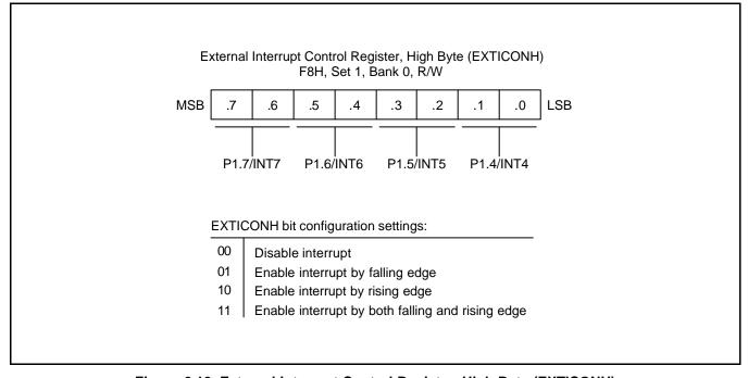
Figure 9-10. External Interrupt Control Register, High Byte (EXTICONH)
