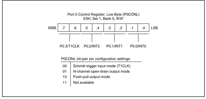
Figure 9-3. Port 0 Low-Byte Control Register (P0CONL)
