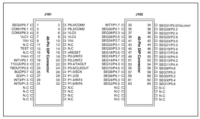
Figure 20-3. 40-Pin Connectors (J101, J102) for TB8275/8/4
