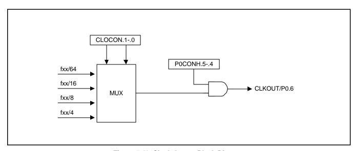
Figure 7-10. Clock Output Block Diagram
