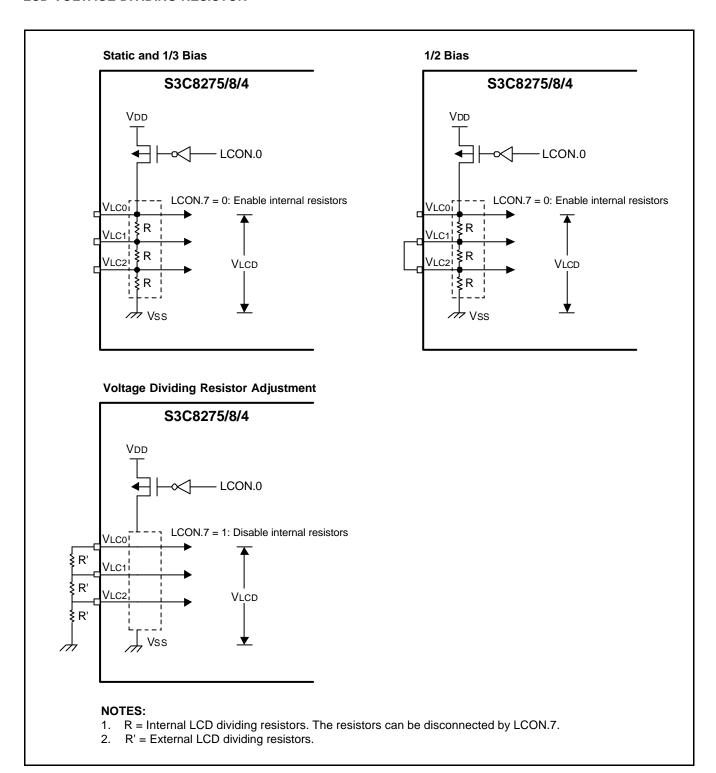
Figure 13-5. Internal Voltage Dividing Resistor Connection
