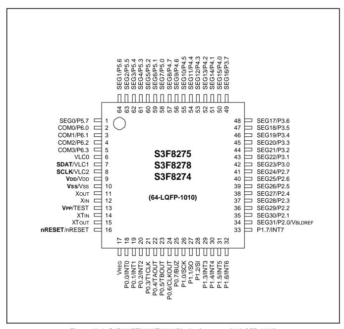
Figure 19-2. S3F8275/F8278/F8274 Pin Assignments (64-LQFP-1010)
