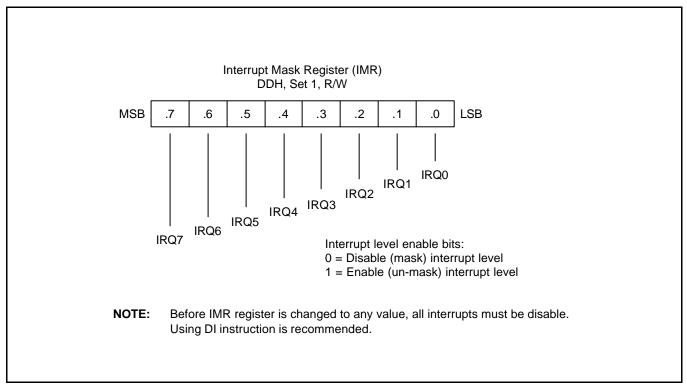
Figure 5-6. Interrupt Mask Register (IMR)
