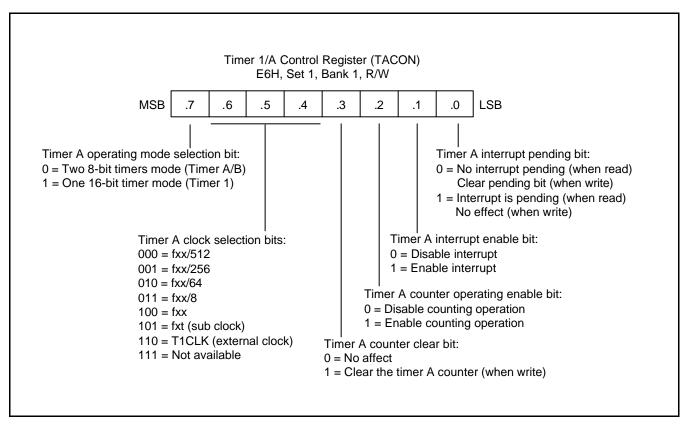
Figure 11-3. Timer 1/A Control Register (TACON)
