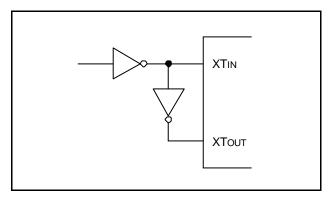
Figure 7-6. External Oscillator (fxt)
