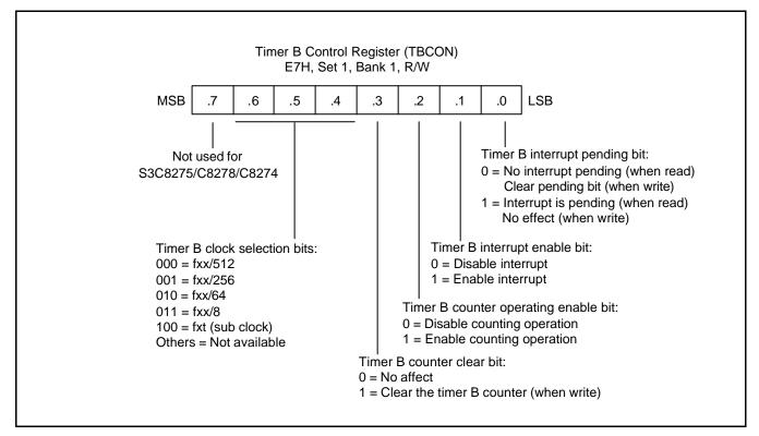
Figure 11-4. Timer B Control Register (TBCON)
