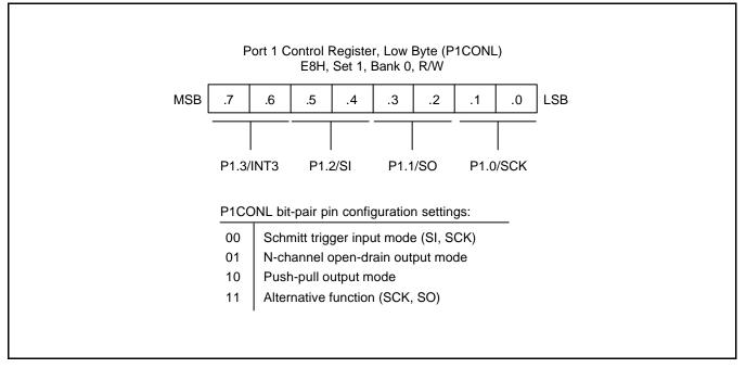
Figure 9-8. Port 1 Low-Byte Control Register (P1CONL)
