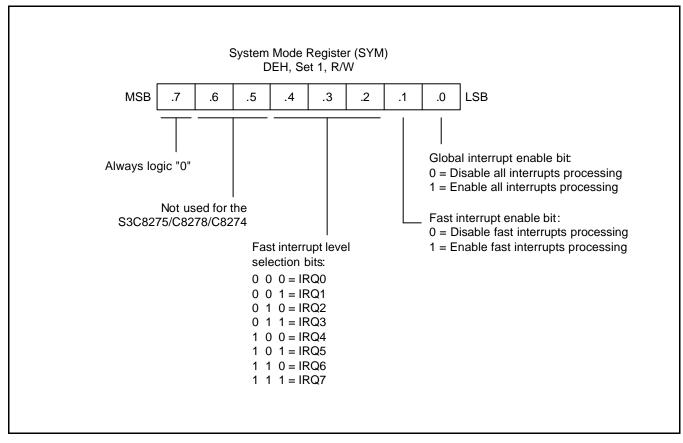
Figure 5-5. System Mode Register (SYM)
