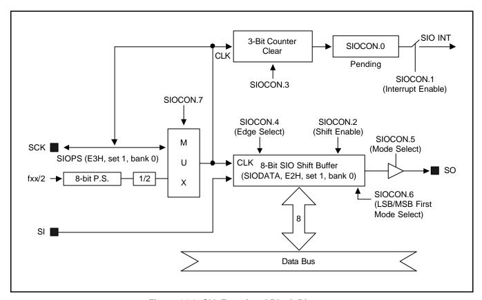
Figure 14-3. SIO Functional Block Diagram
