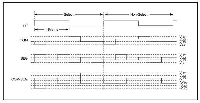
Figure 13-8. Select/No-Select Signal in 1/3 Duty, 1/3 Bias Display Mode
