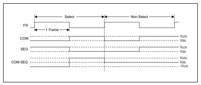
Figure 13-6. Select/No-Select Signals in Static Display Mode
