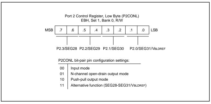
Figure 9-14. Port 2 Low-byte Control Register (P2CONL)
