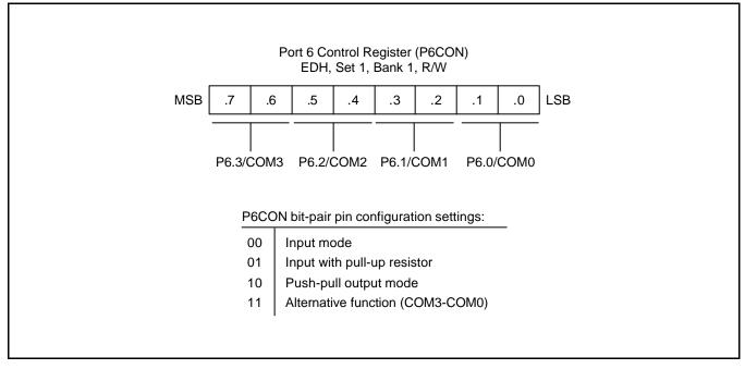
Figure 9-23. Port 6 Control Register (P6CON)
