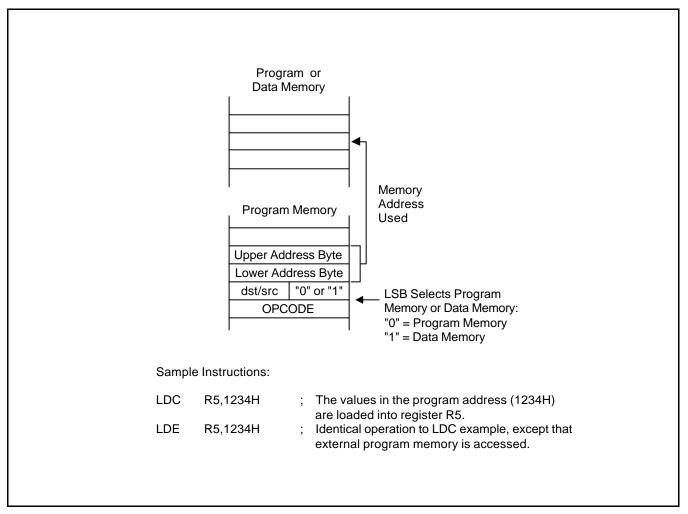
Figure 3-10. Direct Addressing for Load Instructions
