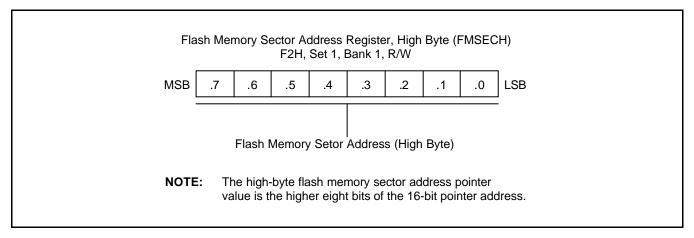
Figure 16-3. Flash Memory Sector Address Register, High Byte (FMSECH)
