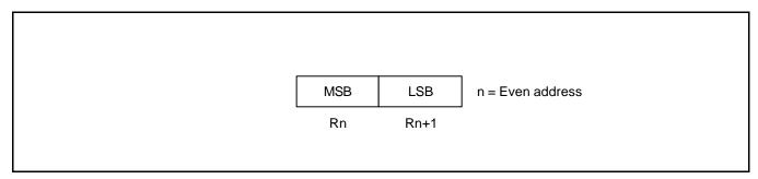
Figure 2-10. 16-Bit Register Pair
