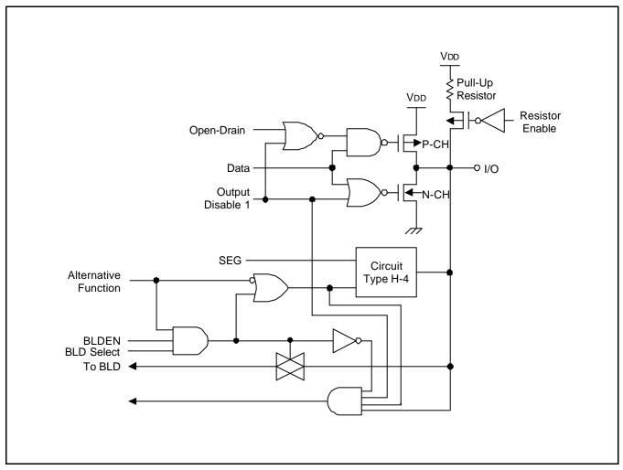
Figure 1-10. Pin Circuit Type H-10 (P2.0)
