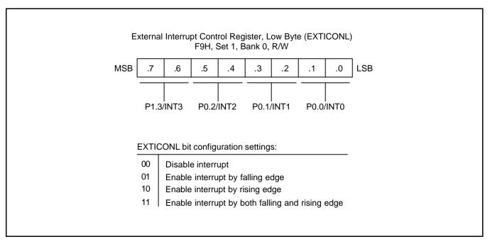
Figure 9-11. External Interrupt Control Register, Low Byte (EXTICONL)
