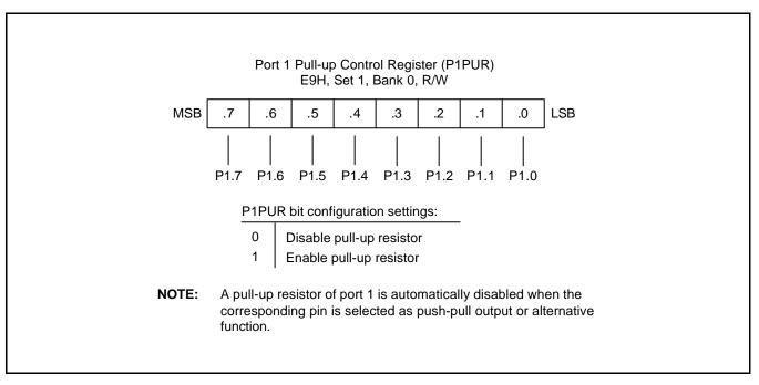
Figure 9-9. Port 1 Pull-up Control Register (P1PUR)
