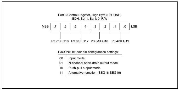
Figure 9-16. Port 3 High Byte Control Register (P3CONH)
