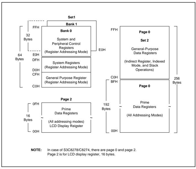
Figure 2-4. Internal Register File Organization (S3C8278/C8274)
