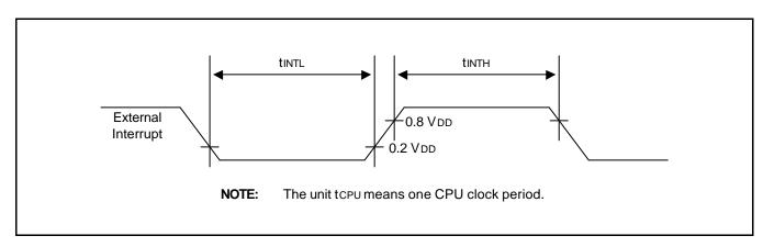
Figure 17-3. Input Timing for External Interrupts
