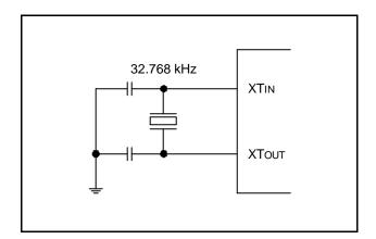
Figure 7-4. Crystal Oscillator (fxt, Normal)
