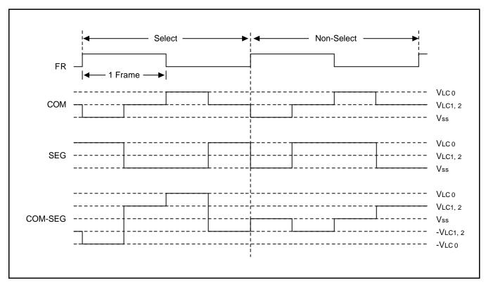
Figure 13-7. Select/No-Select Signal in 1/2 Duty, 1/2 Bias Display Mode
