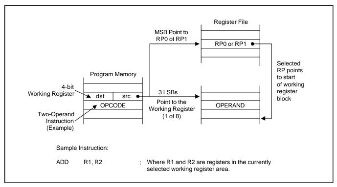
Figure 3-2. Working Register Addressing
