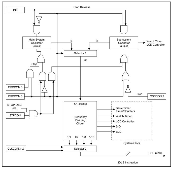
Figure 7-7. System Clock Circuit Diagram
