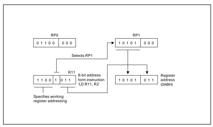
Figure 2-16. 8-Bit Working Register Addressing Example
