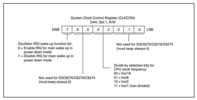
Figure 7-8. System Clock Control Register (CLKCON)
