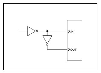
Figure 7-2. External Oscillator (fx)
