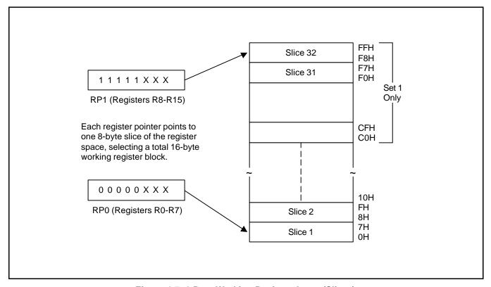
Figure 2-7. 8-Byte Working Register Areas (Slices)
