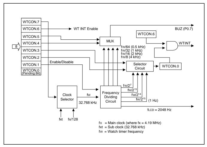
Figure 12-2. Watch Timer Circuit Diagram
