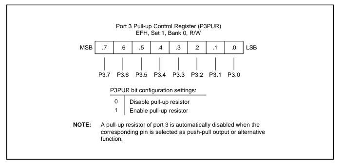
Figure 9-18. Port 3 Pull-up Control Register (P3PUR)
