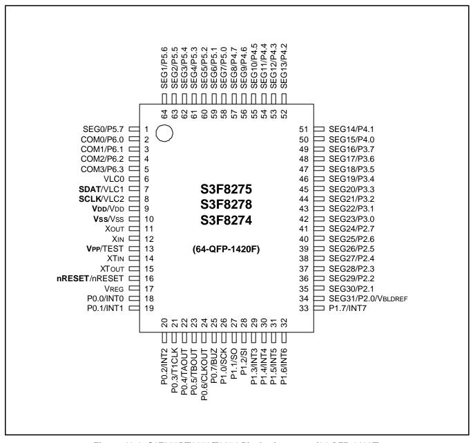
Figure 19-1. S3F8275/F8278/F8274 Pin Assignments (64-QFP-1420F)
