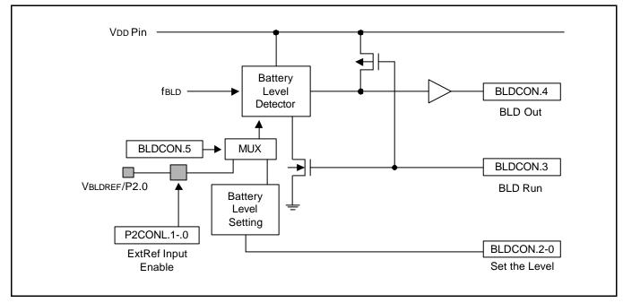
Figure 15-1. Block Diagram for Voltage Level Detect
