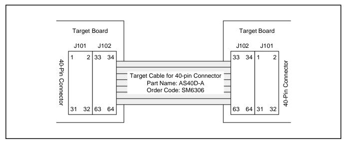
Figure 20-4. S3E8270 Cables for 64-QFP Package
