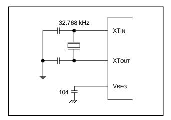
Figure 7-5. Crystal Oscillator (fxt, for Low Current)
