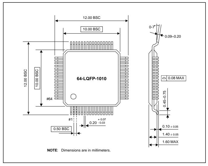
Figure 18-2. 64-Pin LQFP Package Dimensions (64-LQFP-1010)
