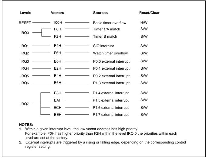
Figure 5-2. S3C8275/C8278/C8274 Interrupt Structure
