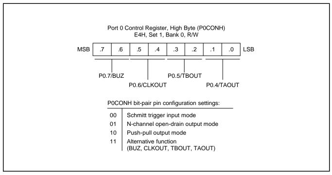
Figure 9-2. Port 0 High-Byte Control Register (P0CONH)
