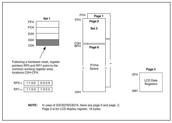
Figure 2-12. Common Working Register Area
