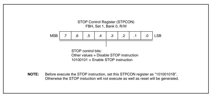
Figure 7-12. STOP Control Register (STPCON)
