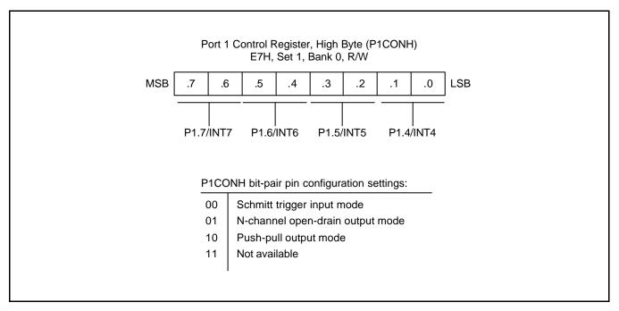
Figure 9-7. Port 1 High-Byte Control Register (P1CONH)
