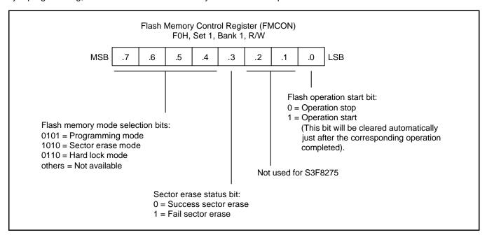
Figure 16-1. Flash Memory Control Register (FMCON)
