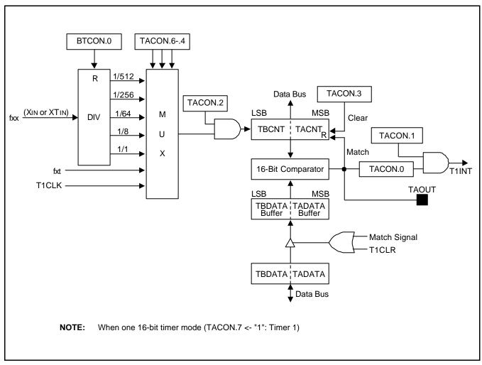
Figure 11-2. Timer 1 Block Diagram (One 16-bit Mode)
