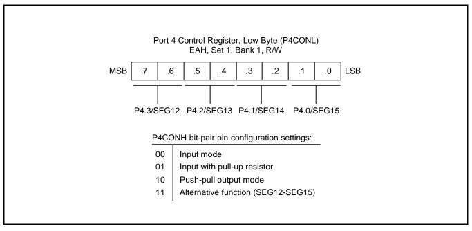
Figure 9-20. Port 4 Low-Byte Control Register (P4CONL)
