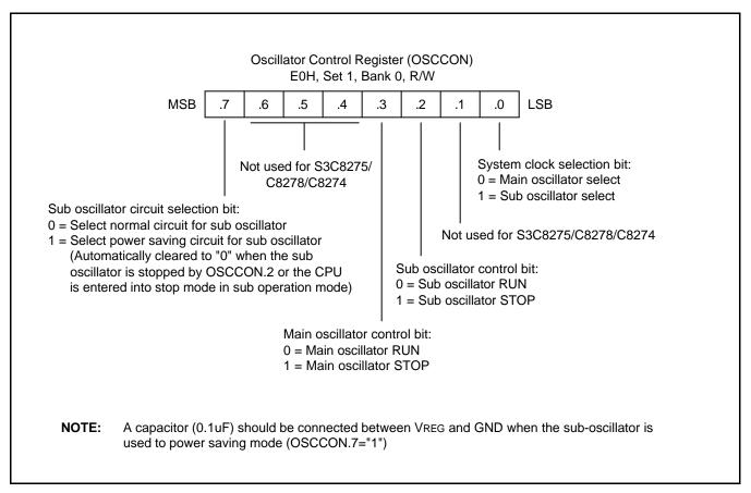
Figure 7-11. Oscillator Control Register (OSCCON)
