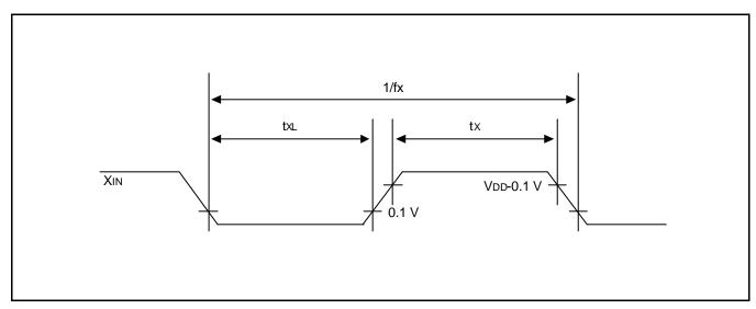
Figure 17-7. Clock Timing Measurement at X<sub>IN</sub>
