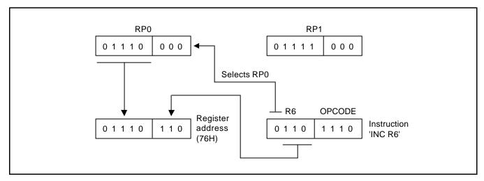
Figure 2-14. 4-Bit Working Register Addressing Example
