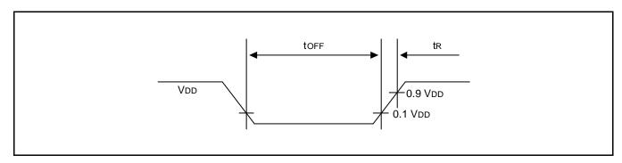
Figure 17-6. LVR (Low Voltage Reset) Timing
