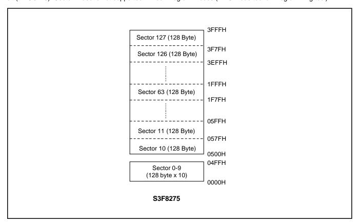
Figure 16-6. Sector Configurations in User Program Mode
