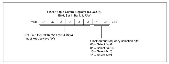
Figure 7-9. Clock Output Control Register (CLOCON)
