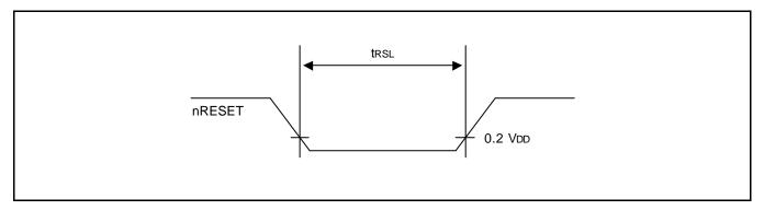
Figure 17-4. Input Timing for RESET
