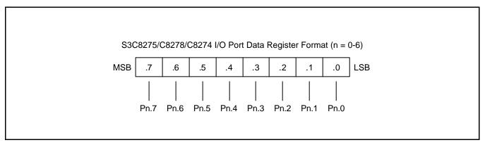
Figure 9-1. S3C8275/C8278/C8274 I/O Port Data Register Format
