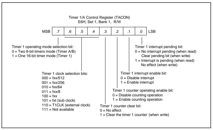
Figure 11-1. Timer 1/A Control Register (TACON)
