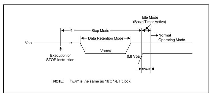
Figure 17-1. Stop Mode Release Timing When Initiated by an External Interrupt
