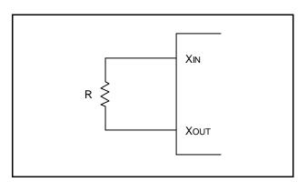
Figure 7-3. RC Oscillator (fx)
