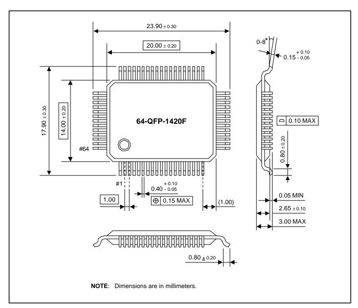
Figure 18-1. 64-Pin QFP Package Dimensions (64-QFP-1420F)
