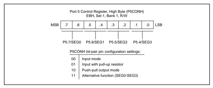
Figure 9-21. Port 5 High-Byte Control Register (P5CONH)
