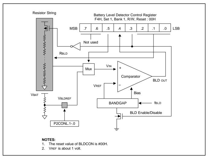
Figure 15-2. Battery Level Detect Circuit and Control Register
