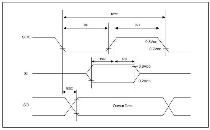
Figure 17-5. Serial Data Transfer Timing
