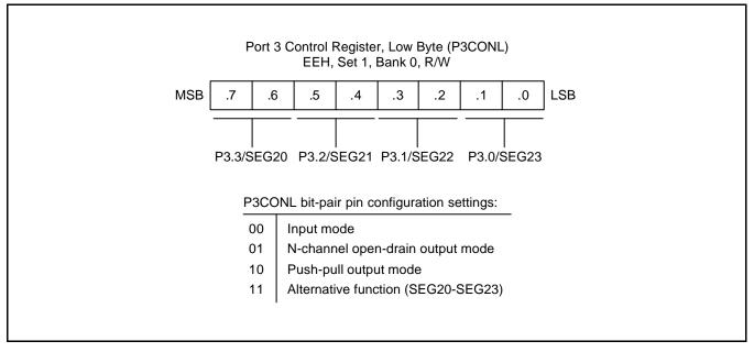
Figure 9-17. Port 3 Low Byte Control Register (P3CONL)
