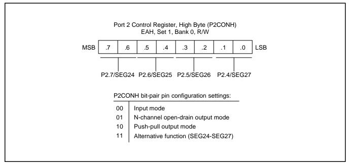
Figure 9-13. Port 2 High-byte Control Register (P2CONH)
