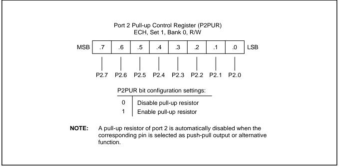
Figure 9-15. Port 2 Pull-up Control Register (P2PUR)
