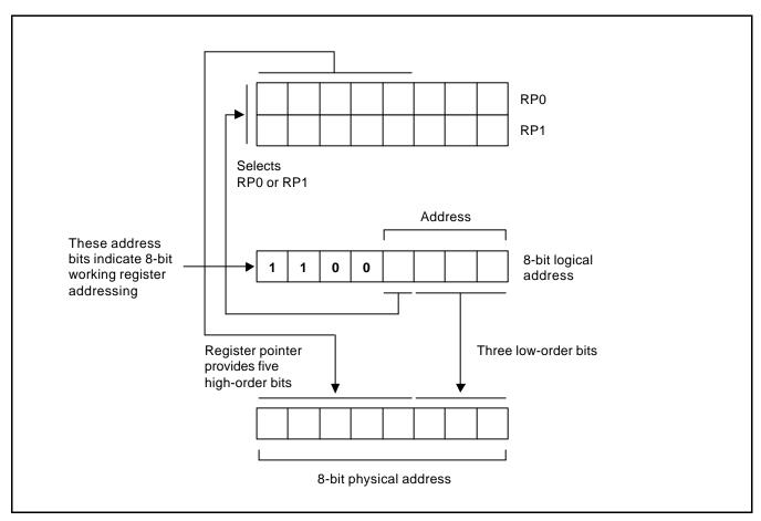
Figure 2-15. 8-Bit Working Register Addressing
