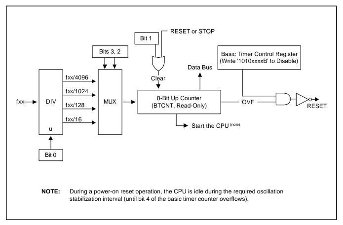
Figure 10-2. Basic Timer Block Diagram
