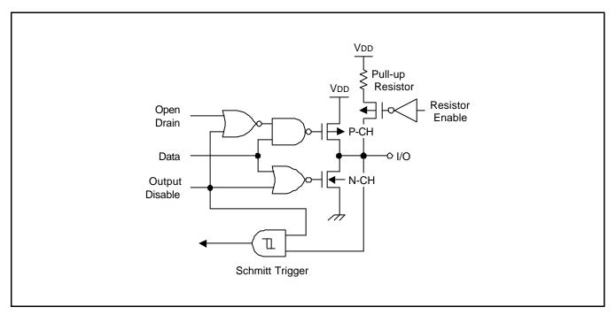
Figure 1-6. Pin Circuit Type E-4 (P0, P1)
