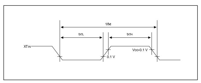
Figure 17-8. Clock Timing Measurement at  $\mathrm{XT}_{\mathrm{IN}}$
