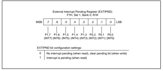
Figure 9-12. External Interrupt Pending Register (EXTIPND)
