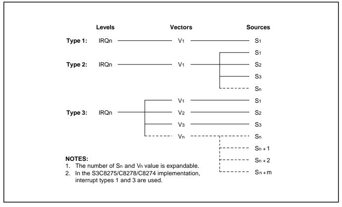
Figure 5-1. S3C8-Series Interrupt Types
