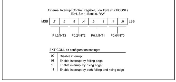
Figure 9-5. External Interrupt Control Register, Low Byte (EXTICONL)
