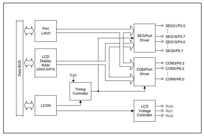
Figure 13-2. LCD Circuit Diagram
