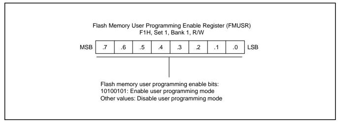
Figure 16-2. Flash Memory User Programming Enable Register (FMUSR)
