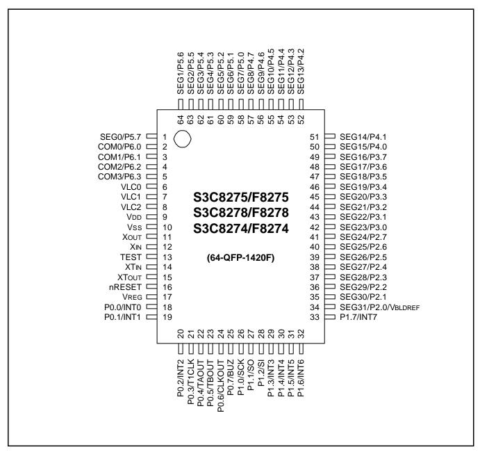
Figure 1-2. S3C8275/F8275/C8278/F8278/C8274/F8274 Pin Assignments (64-QFP-1420F)
