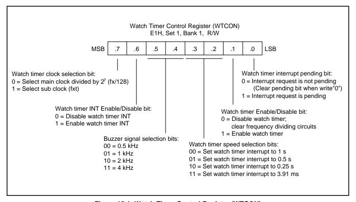
Figure 12-1. Watch Timer Control Register (WTCON)
