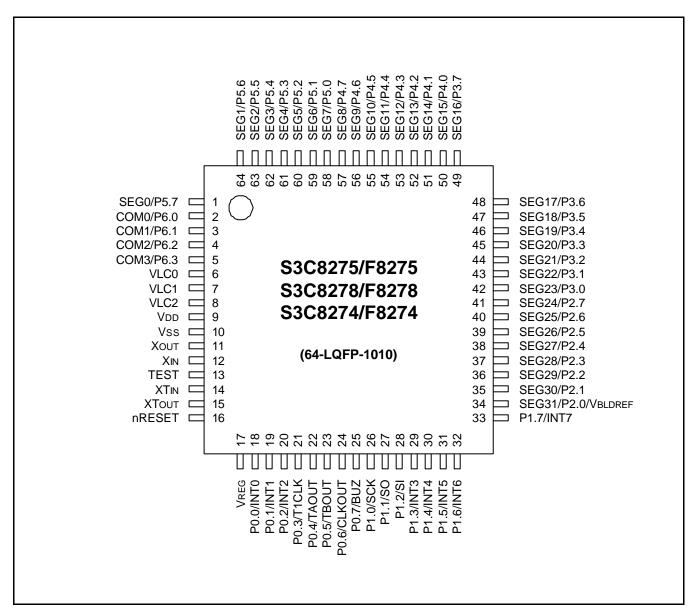
Figure 1-3. S3C8275/F8275/C8278/F8278/C8274/F8274 Pin Assignments (64-LQFP-1010)
