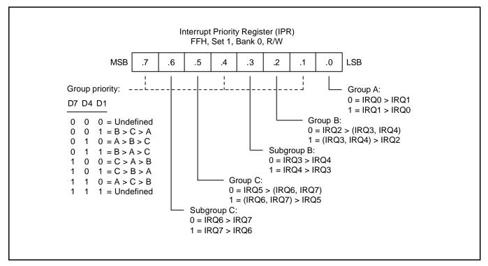
Figure 5-8. Interrupt Priority Register (IPR)
