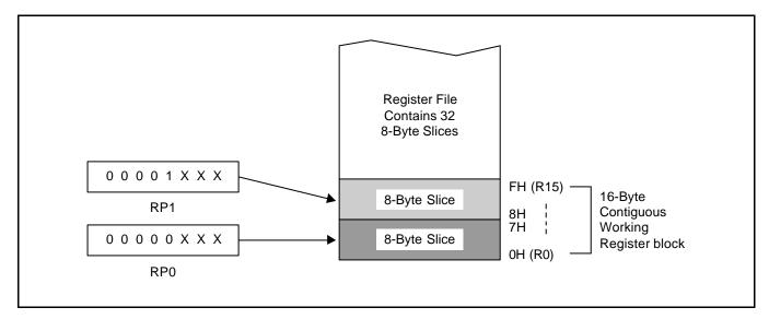
Figure 2-8. Contiguous 16-Byte Working Register Block
