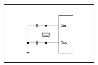
Figure 7-1. Crystal/Ceramic Oscillator (fx)
