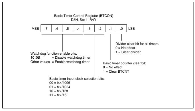
Figure 10-1. Basic Timer Control Register (BTCON)
