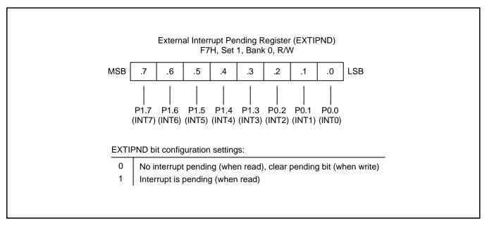
Figure 9-6. External Interrupt Pending Register (EXTIPND)
