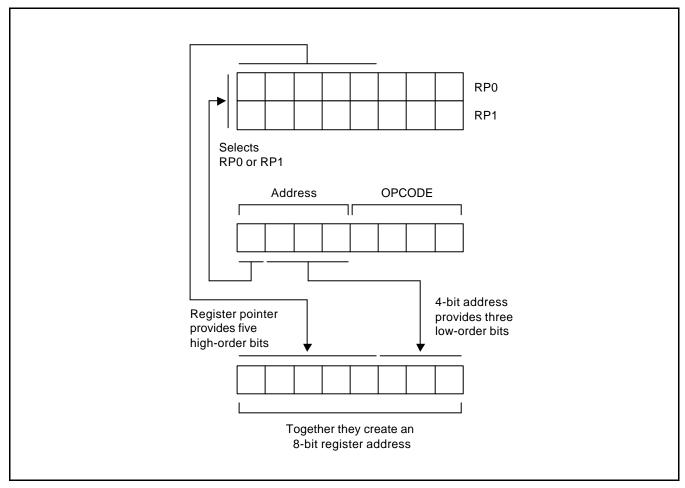
Figure 2-13. 4-Bit Working Register Addressing
