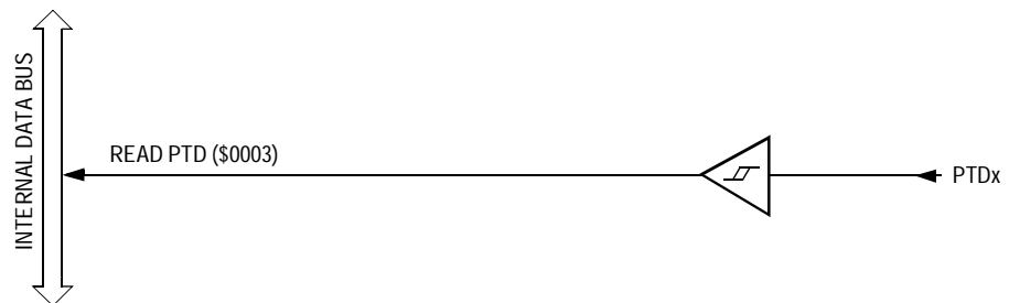
Figure 15-12. Port D Input Circuit
