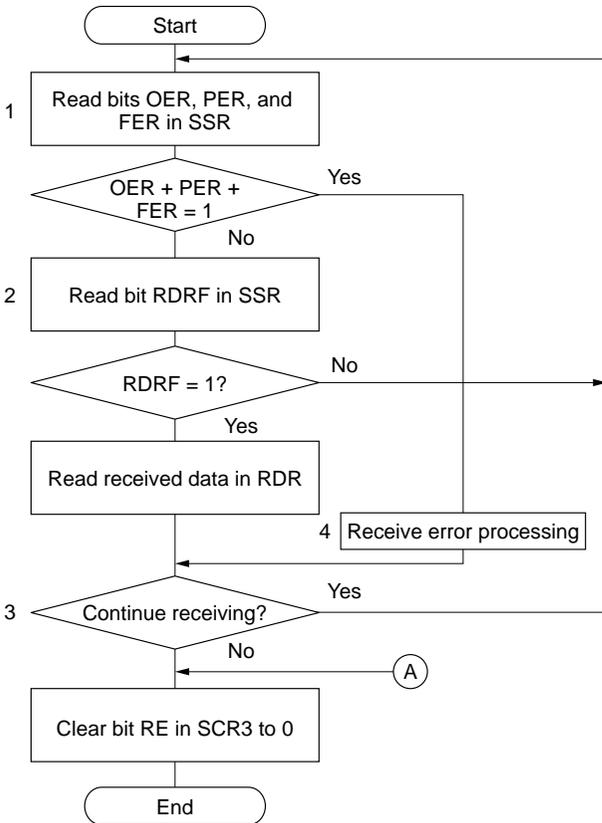
1. Read bits OER, PER, and FER in the serial status register (SSR) to determine if a receive error has occurred. If a receive error has occurred, receive error processing is executed.
