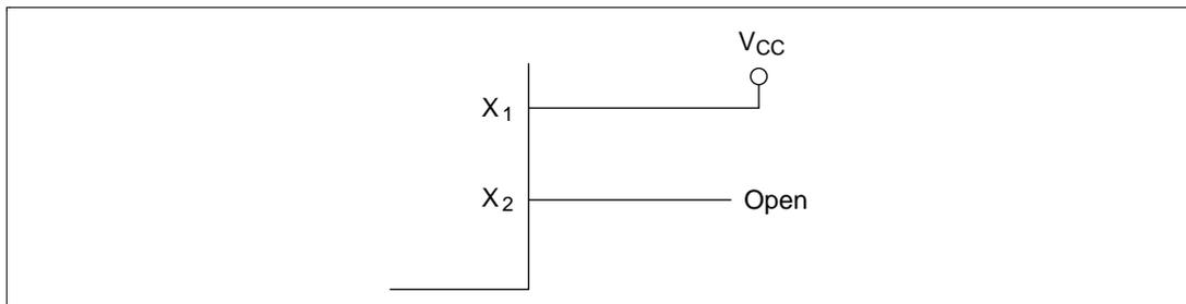
**Figure 4.9 Pin Connection when Not Using Subclock**
