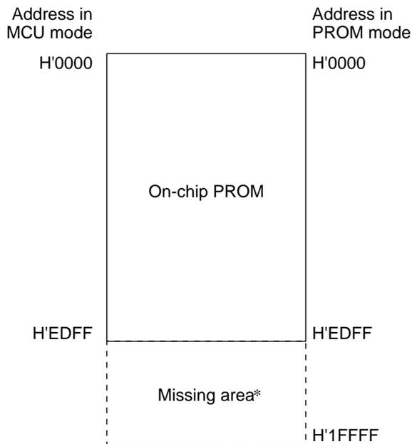
Note: \* If read in PROM mode, this address area returns unpredictable output data. When programming with a PROM programmer, be sure to specify addresses from H'0000 to H'EDFF. If address H'EE00 and higher addresses are programmed by mistake, it may become impossible to program the PROM or verify the programmed data. When programming, assign H'FF data to this address area (H'EE00 to H'1FFFF).
