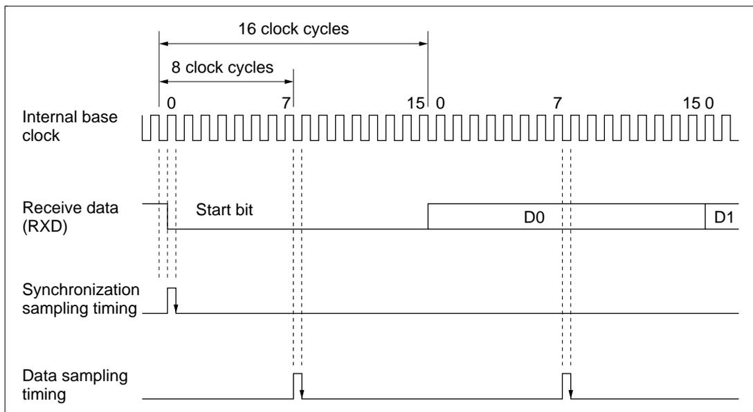
**Figure 10.27 Receive Data Sampling Timing in Asynchronous Mode**
