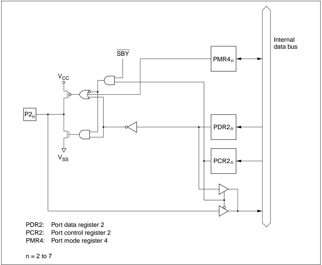
Figure C.2 (a) Port 2 Block Diagram (Pins P2<sub>7</sub> to P2<sub>2</sub>)
