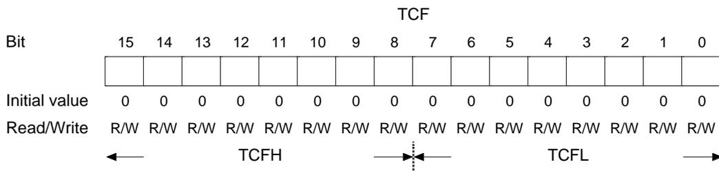
TCF is a 16-bit read/write up-counter consisting of two cascaded 8-bit timer counters, TCFH and TCFL. TCF can be used as a 16-bit counter, with TCFH as the upper 8 bits and TCFL as the lower 8 bits of the counter, or TCFH and TCFL can be used as independent 8-bit counters.
