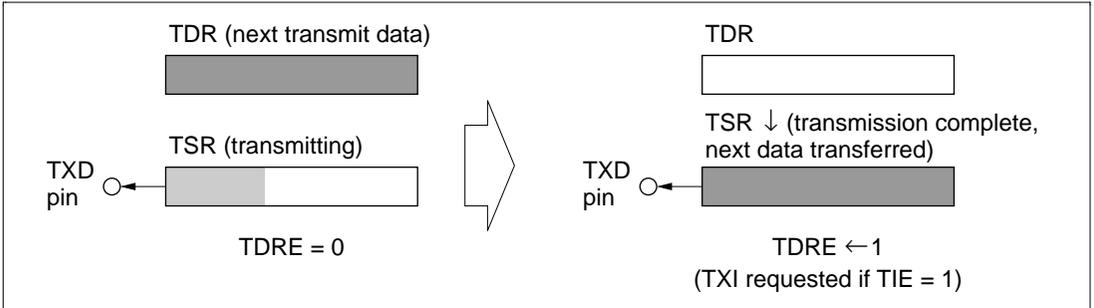
**Figure 10.8 (b) TDRE Setting and TXI Interrupt**
