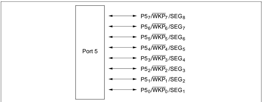
**Figure 8.5 Port 5 Pin Configuration**
