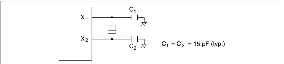
**Figure 4.7 Typical Connection to 32.768-kHz Crystal Oscillator**
