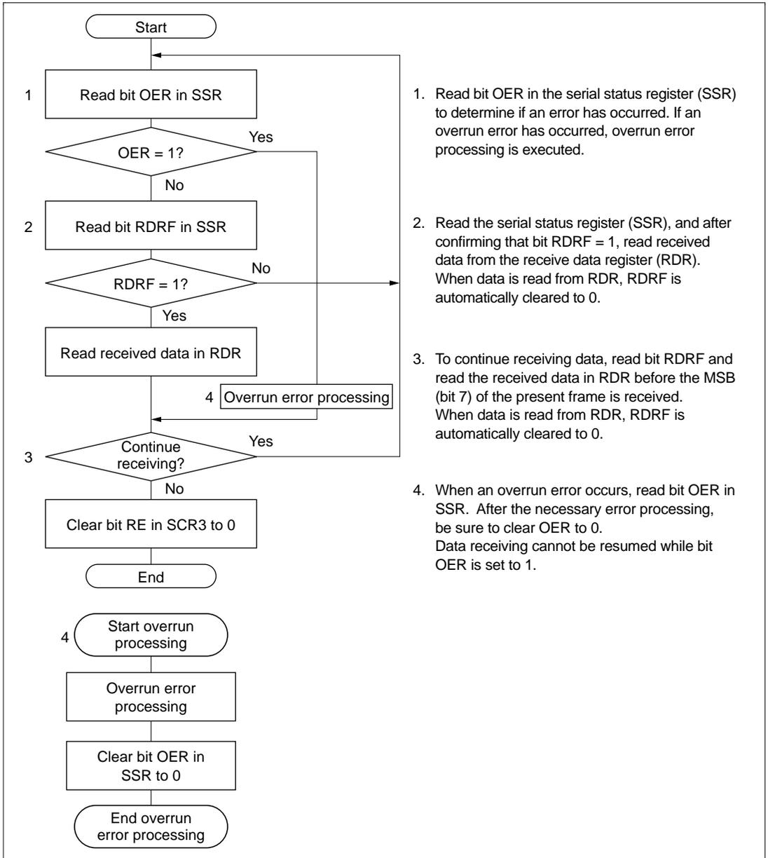
1. Read bit OER in the serial status register (SSR) to determine if an error has occurred. If an overrun error has occurred, overrun error processing is executed.
