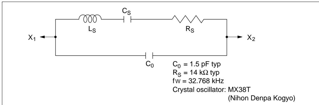
**Figure 4.8 Equivalent Circuit of 32.768-kHz Crystal Oscillator**
