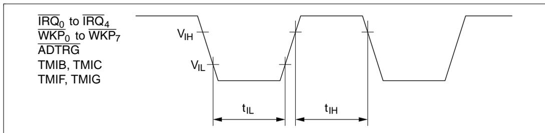
Figure 14.3 Input Timing
