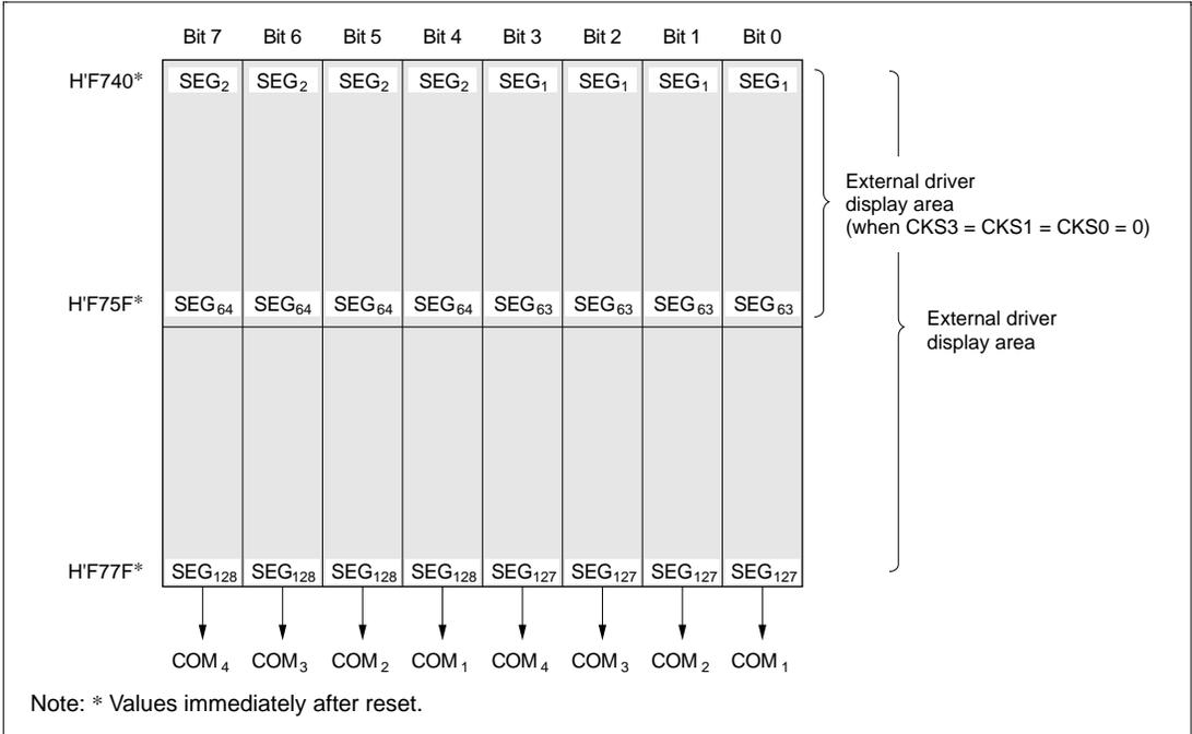
**Figure 13.11 LCD RAM Map When All External Segments are Used**
