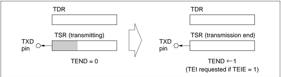
**Figure 10.8 (c) TEND Setting and TEI Interrupt**
