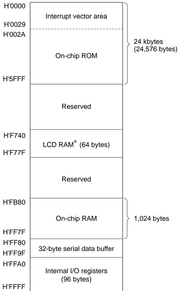
Note: \* The LCD RAM addresses are the addresses after a reset.
