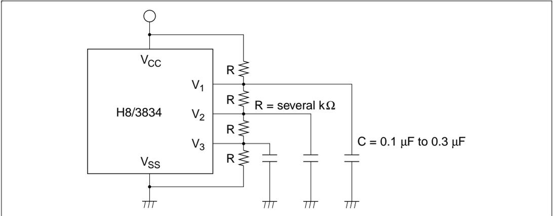
**Figure 13.14** Connecting an External Resistive Voltage Divider
