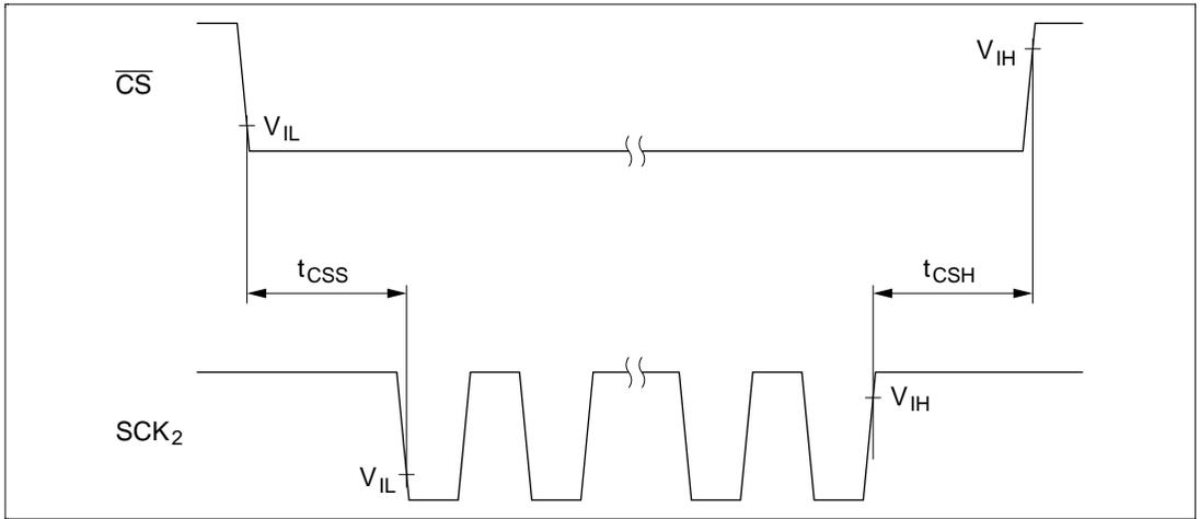
**Figure 14.6 Serial Interface 2 Chip Select Timing**
