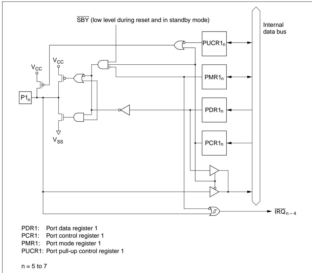
Figure C.1 (a) Port 1 Block Diagram (Pins P1<sub>7</sub> to P1<sub>5</sub>)
