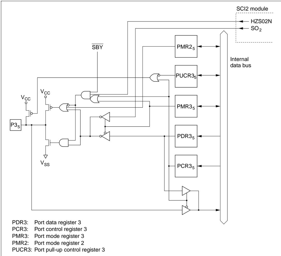
**Figure C.3 (c) Port 3 Block Diagram (Pin P3<sub>5</sub>)**
