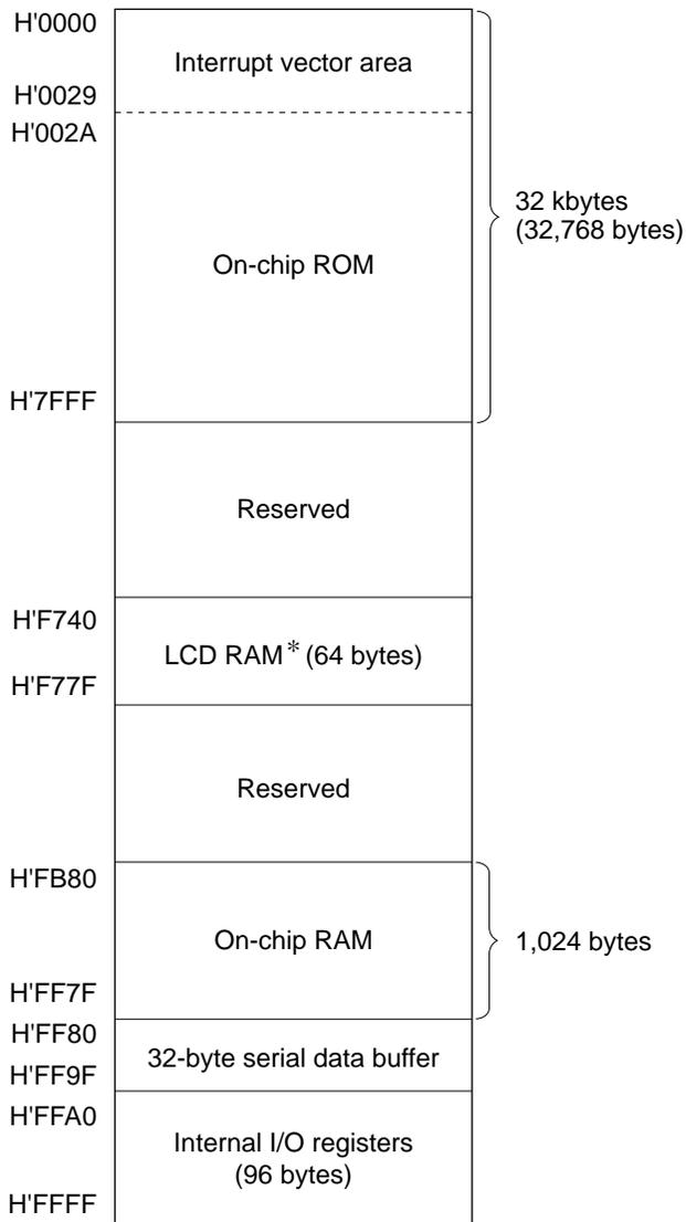
Note: \* The LCD RAM addresses are the addresses after a reset.
