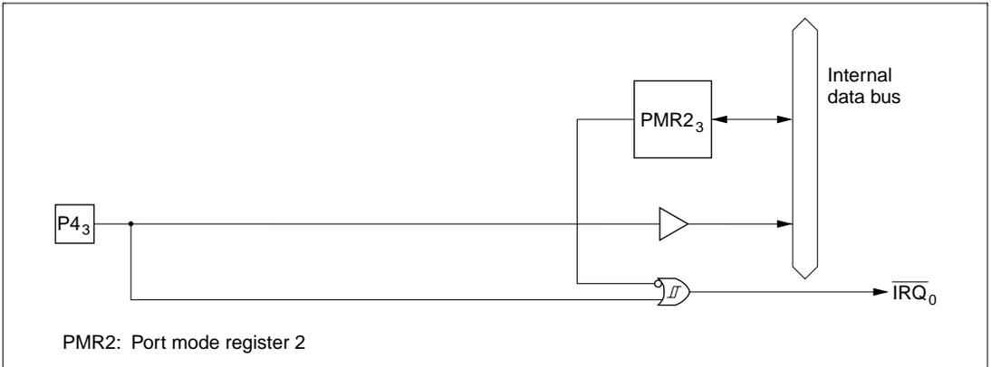
**Figure C.4 (a) Port 4 Block Diagram (Pin P4<sub>3</sub>)**
