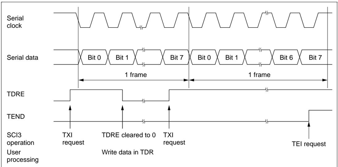
**Figure 10.18 Typical SCI3 Transmit Operation in Synchronous Mode**
