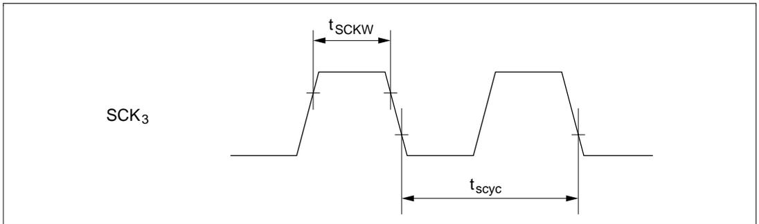
**Figure 14.7 SCK<sub>3</sub> Input Clock Timing**
