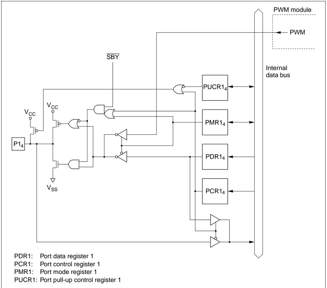
**Figure C.1 (b) Port 1 Block Diagram (Pin P1<sub>4</sub>)**
