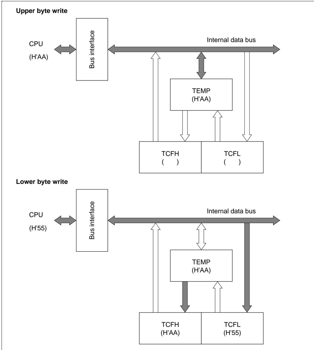
**Figure 9.5 TCF Write Operation (CPU → TCF)**
