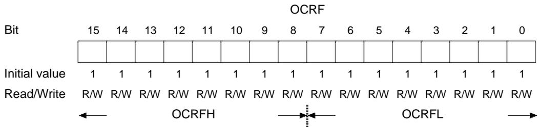
OCRF is a 16-bit read/write output compare register consisting of two 8-bit read/write registers OCRFH and OCRFL. It can be used as a 16-bit output compare register, with OCRFH as the upper 8 bits and OCRFL as the lower 8 bits of the register, or OCRFH and OCRFL can be used as independent 8-bit registers.
