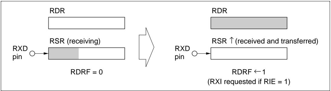
**Figure 10.8 (a) RDRF Setting and RXI Interrupt**
