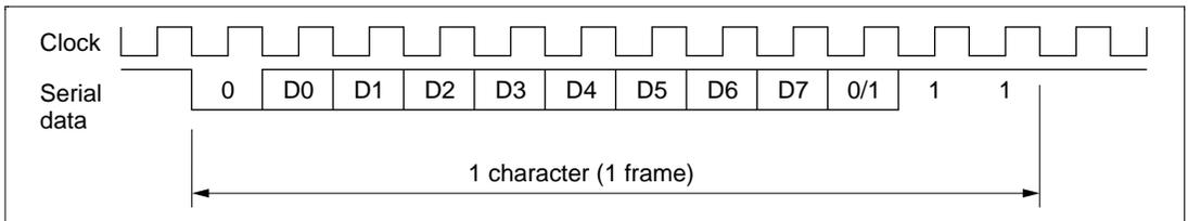
**Figure 10.10 Phase Relation of Output Clock and Communication Data in Asynchronous Mode (8-Bit Data, Parity Bit Added, and 2 Stop Bits)**
