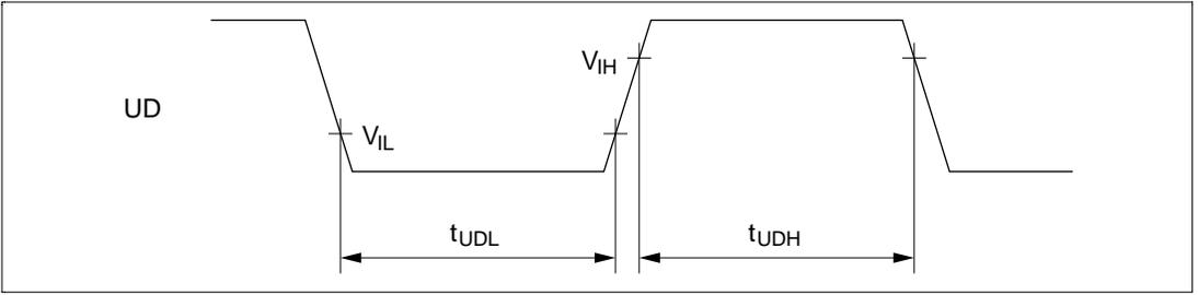
**Figure 14.4 UD Pin Minimum Transition Width Timing**
