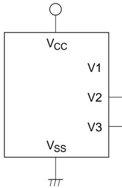
**Figure 13.2 LCD Driver Power Supply Processing at 1/2 Duty**
