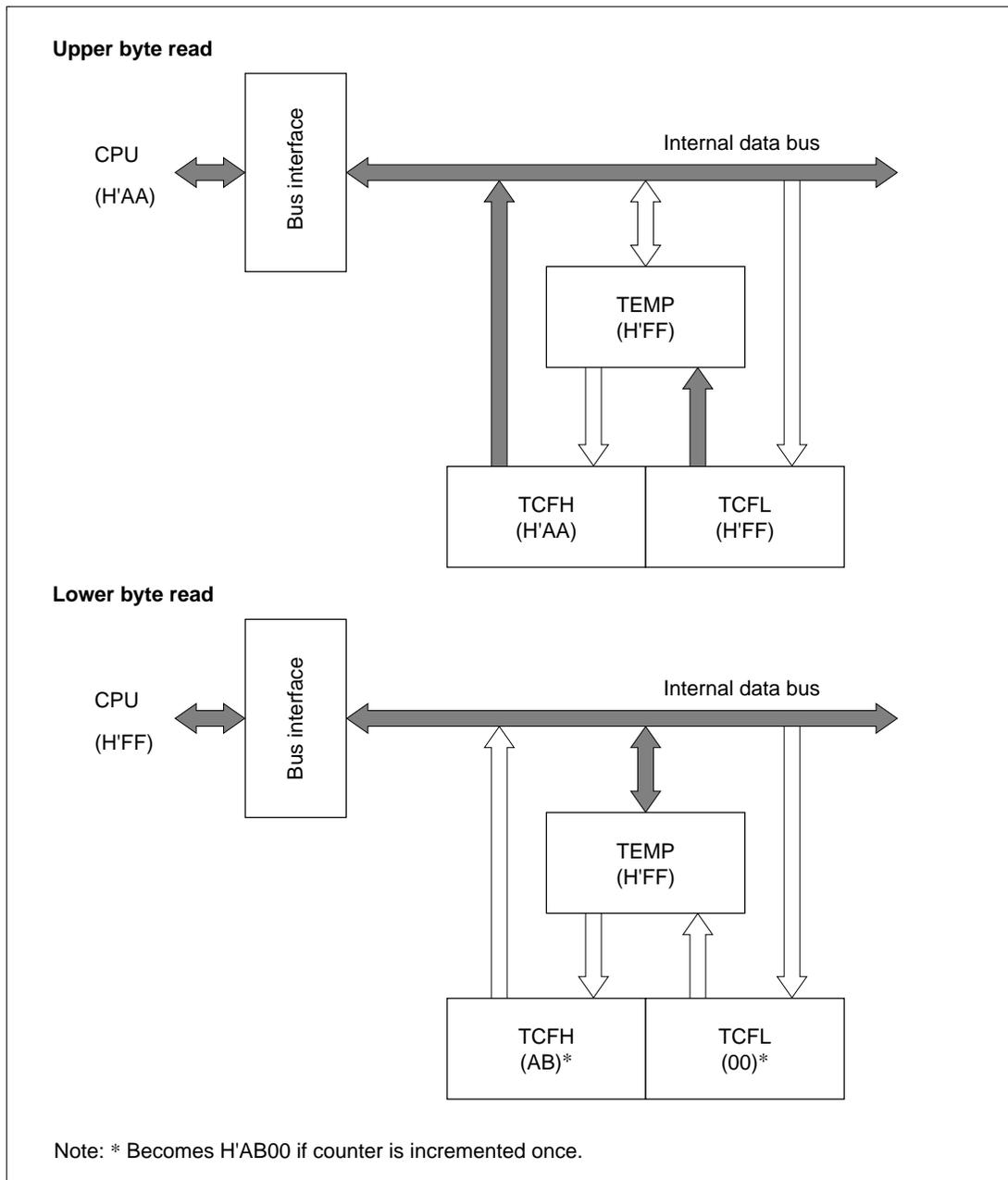
**Figure 9.6 TCF Read Operation (TCF → CPU)**
