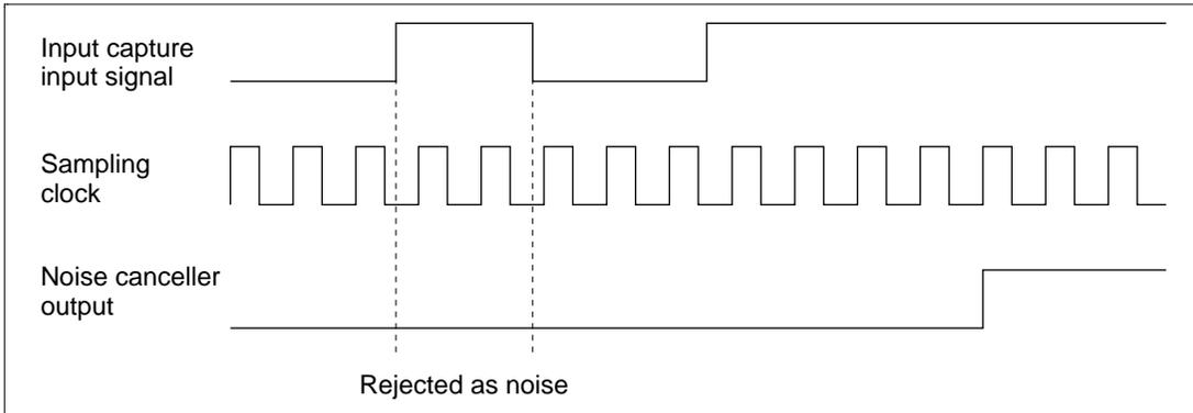
**Figure 9.10 Noise Canceller Circuit Timing (Example)**
