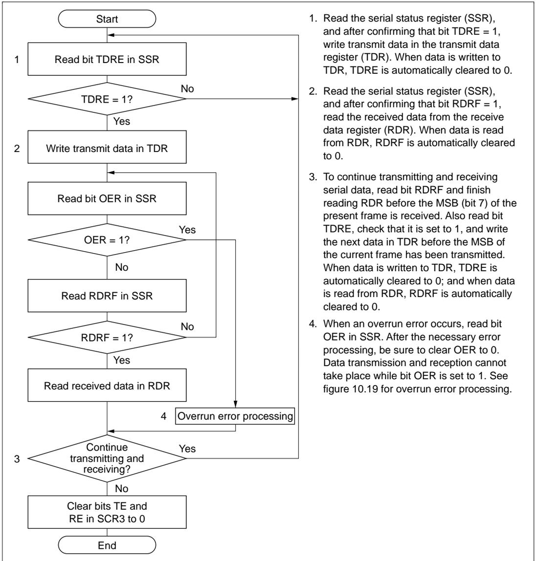
1. Read the serial status register (SSR), and after confirming that bit TDRE = 1, write transmit data in the transmit data register (TDR). When data is written to TDR, TDRE is automatically cleared to 0.
