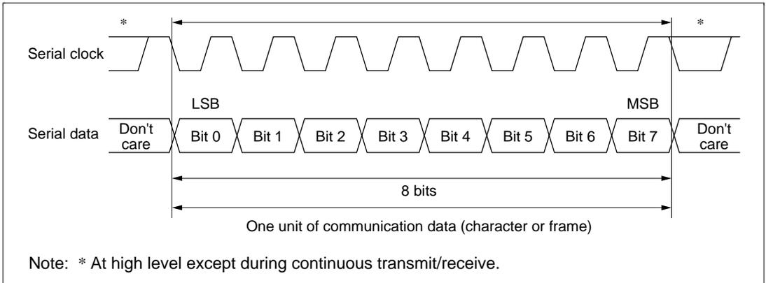
**Figure 10.16 Data Format in Synchronous Communication Mode**
