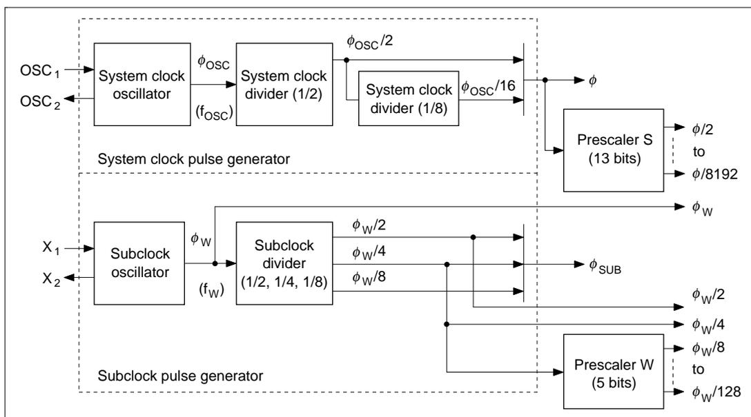
Figure 4.1 Block Diagram of Clock Pulse Generators
