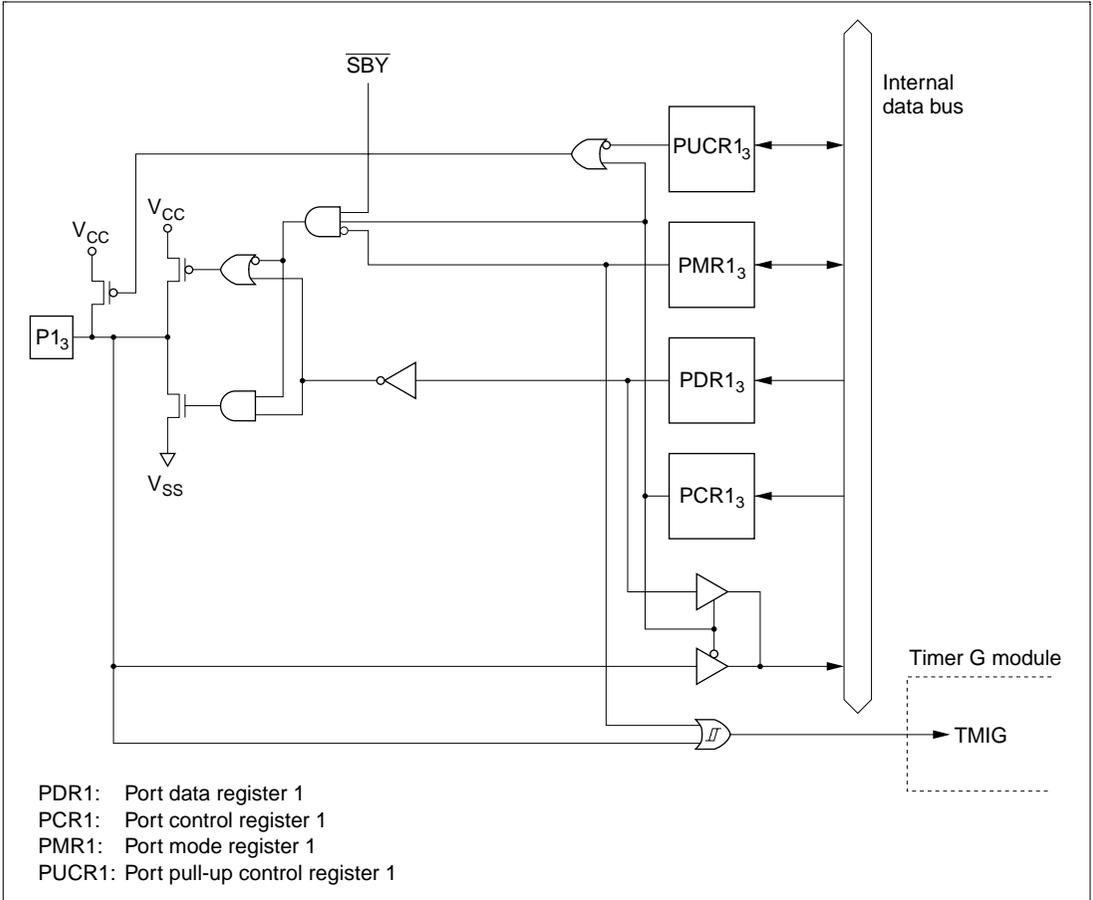
**Figure C.1 (c) Port 1 Block Diagram (Pin P1<sub>3</sub>)**
