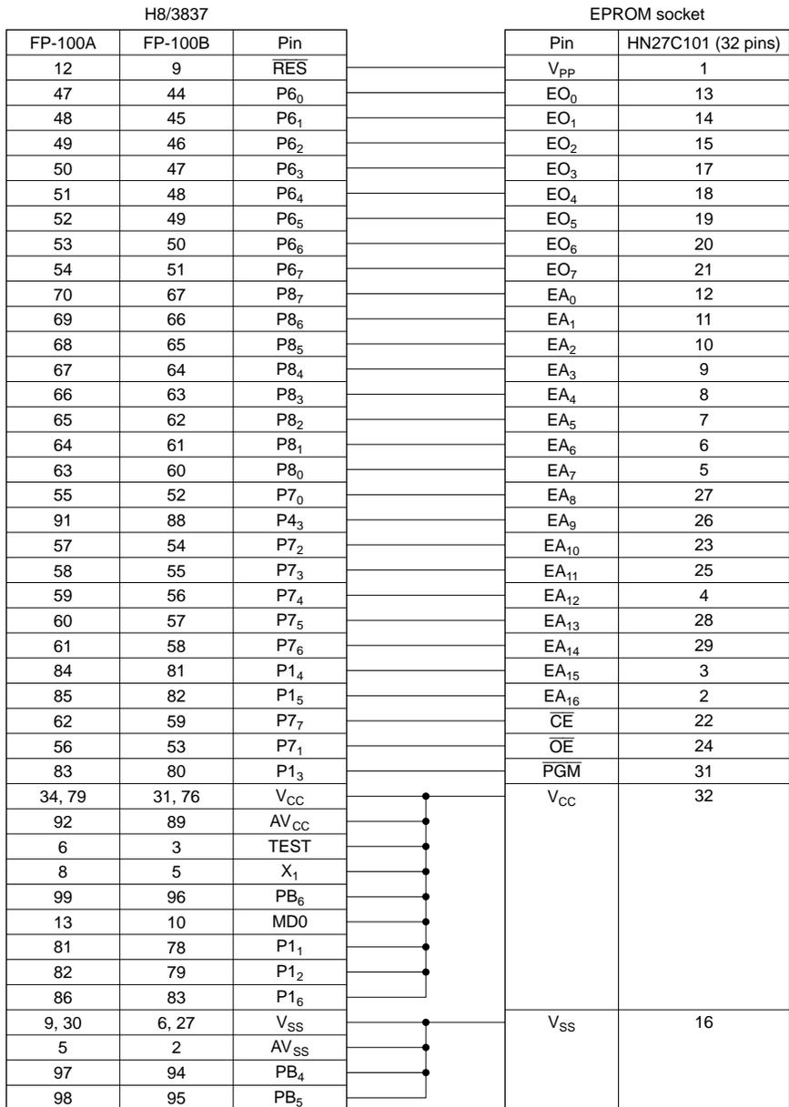
Note: Pins not indicated in the figure should be left open.
