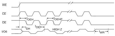
Notes: 1. Toggling either  $\overline{\text{OE}}$  or  $\overline{\text{CE}}$  or both  $\overline{\text{OE}}$  and  $\overline{\text{CE}}$  will operate toggle bit. The t<sub>OEHP</sub> specification must be met by the toggling input(s).
