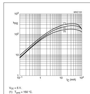
Fig.3 DC current gain as a function of collector current; typical values.
