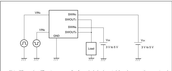
Note: When using different power supplies for a single load, control them by connecting an external capacitor so that both switches are not ON at the same time.
