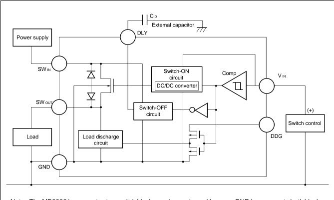
Note: The MB3802 incorporates two switch blocks as shown above. However, GND is common to both blocks.
