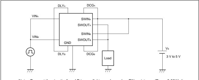
Note: Connect the circuits A and B in parallel to produce a low ON resistance (Ron =  $0.06\Omega$ ). In this case, connect the DLYA and DLYB pins in common to give synchronous ON/OFF between both switches.
