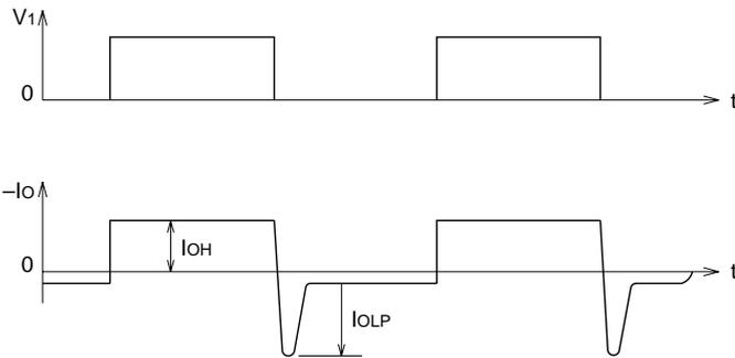
**Note:** IOH and IOLP correspond to base forward current IB1 and base reverse current IB2 of the transistor modules to be driven respectively.
