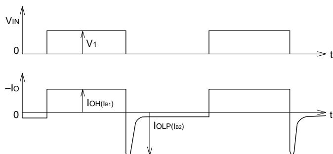
**Note:**  $I_{OH}$  and  $I_{OLP}$  correspond to base forward current  $I_{b1}$  and base reverse current  $I_{b2}$  of the transistor modules to be driven respectively.
