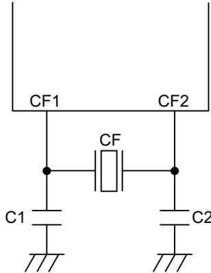
Figure 1 Ceramic Oscillation Circuit.
