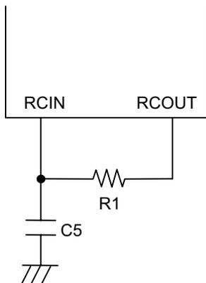
Figure 3 RC Oscillation Circuit.
