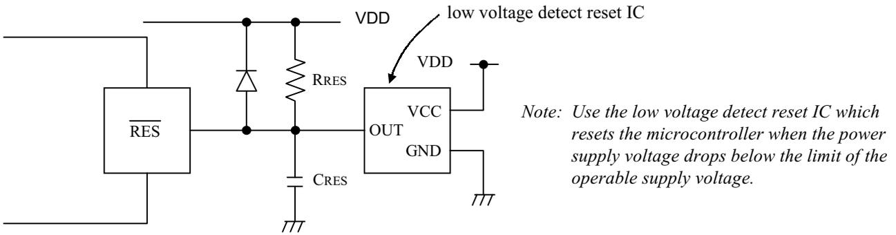
Figure 4 Reset Circuit.
