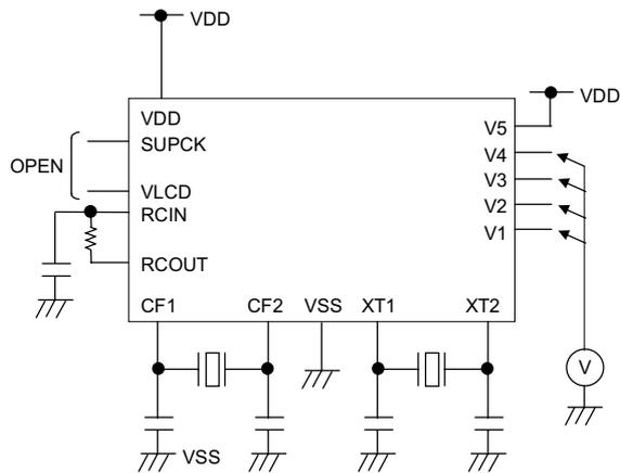
Figure 9 V1 - V4 Terminal Output Voltage Measurement Circuit.
