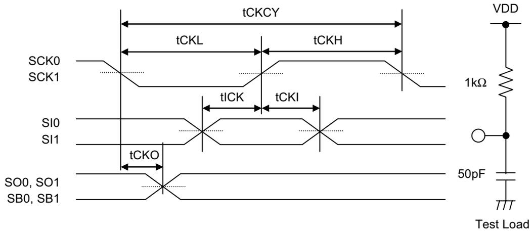
Figure 5 Serial Input Test Condition.
