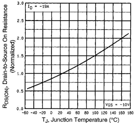
**Fig 4.** Normalized On-Resistance
