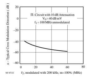
Figure 3. Typ. Cross Modulation Distortion vs. Frequency  ${\rm f}_2$
