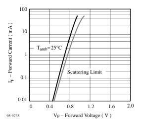
Figure 1. Forward Current vs. Forward Voltage
