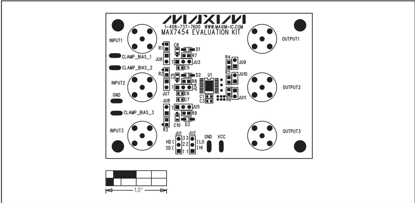
Figure 2. MAX7454 EV Kit Component Placement Guide—Component Side
