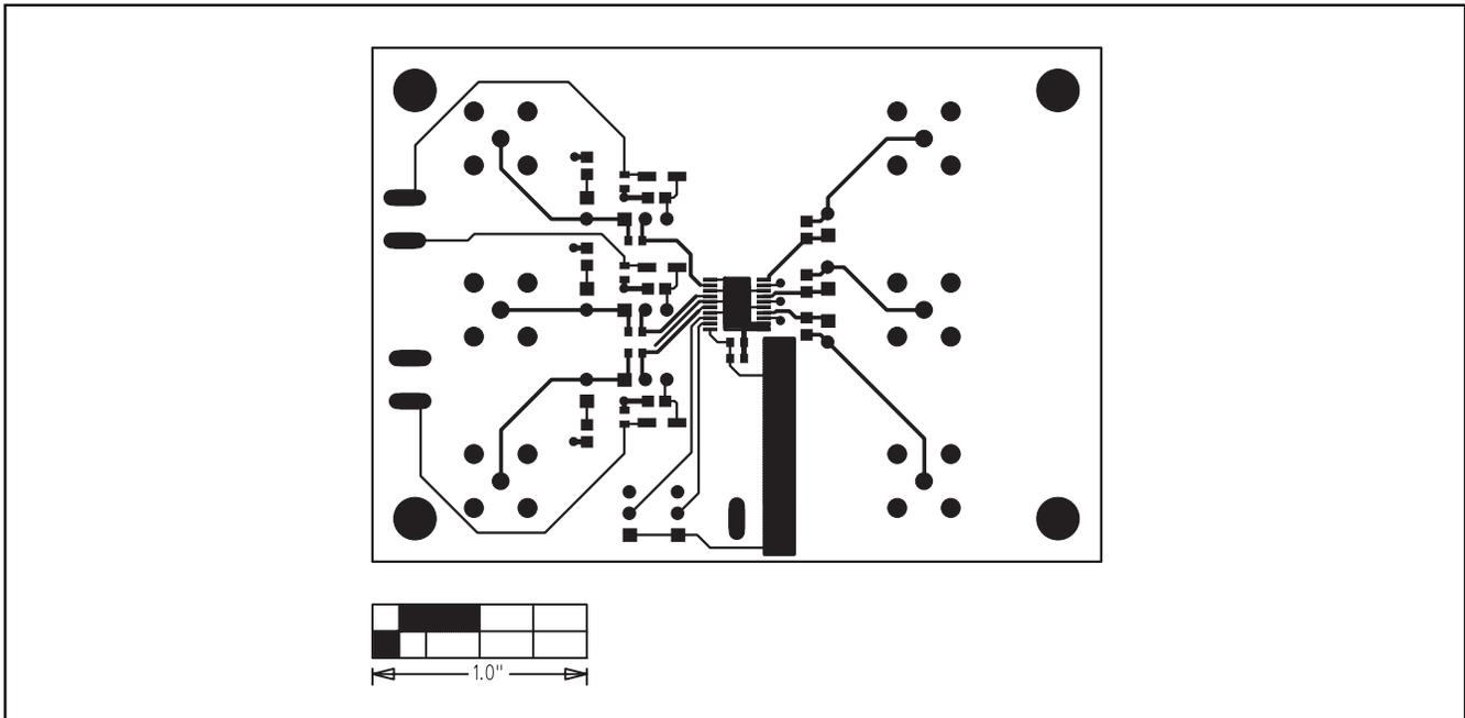
Figure 3. MAX7454 EV Kit PC Board Layout—Component Side
