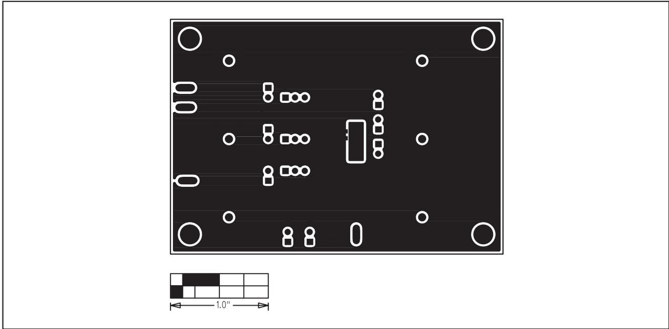
Figure 4. MAX7454 EV Kit PC Board Layout—Solder Side
