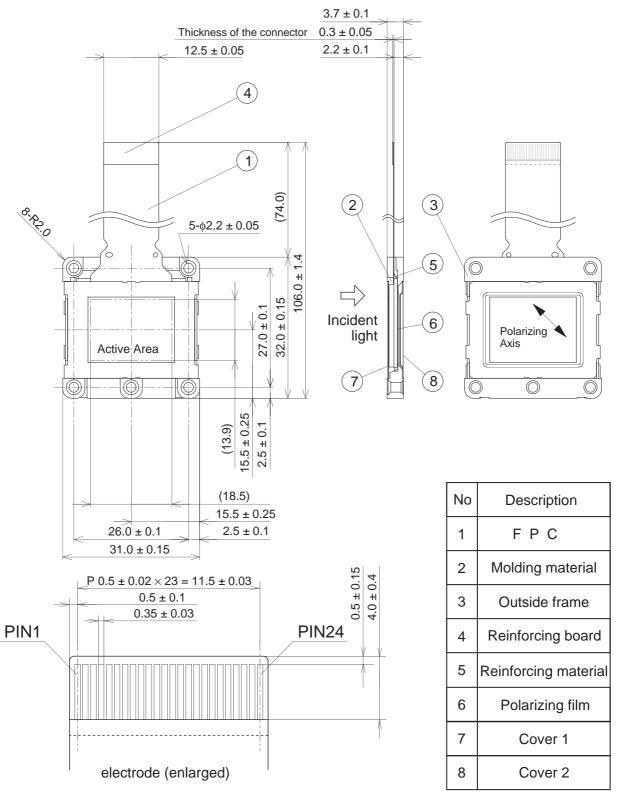
The rotation angle of the active area relative to H and V is  $\pm$  1°.
