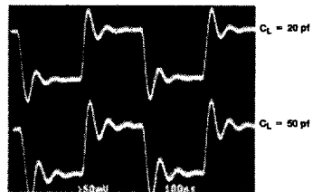
Pulse Response with V+ = 3V, V- = -2V
