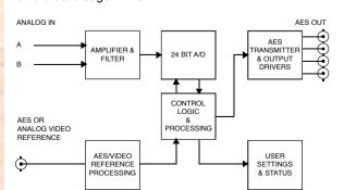
For 48 kHz AES, the RossGear ADC-8532 is capable of referencing to either an external analog video or AES (DARS) reference. Referencing to the external AES reference guarantees a properly phased AES output.
