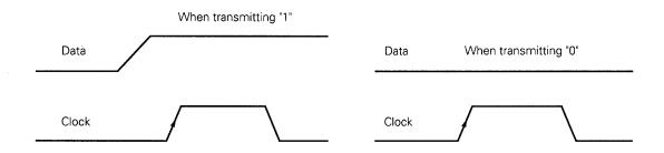
Display data are shifted from the 48th bit in order, and data transmission finishes when the 1st bit (LSB) Display datum is transmitted.
