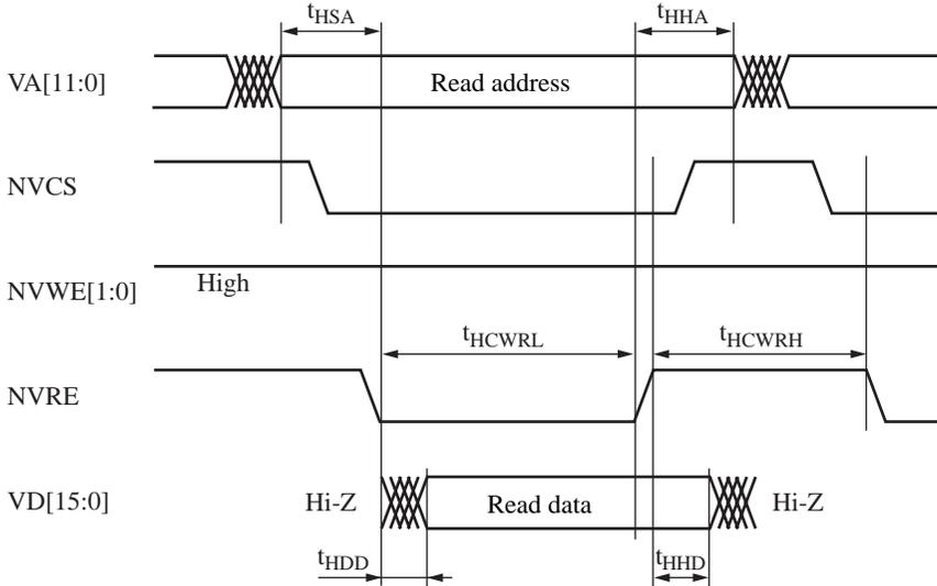
Figure 8. Host memory and register read timing
