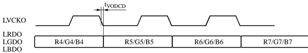
Figure 6. Horizontal timing (When V\_POS = 1)
