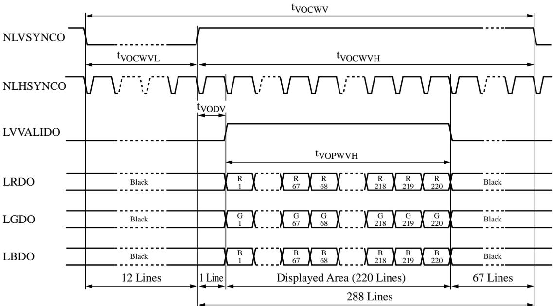
Note) When V\_POS = 1, line 0 and lines 221 to 287 will be filled with black in the LCD RGB, and only lines 1 to 220 will be output.
