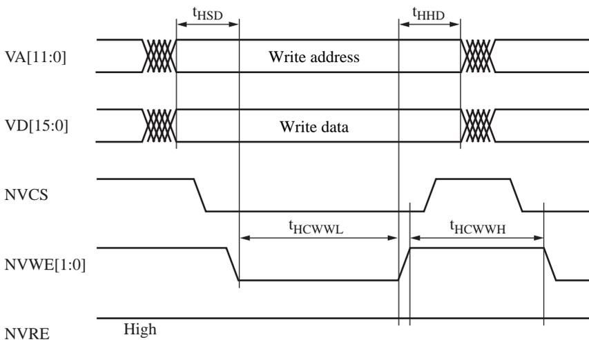
Figure 7. Host memory and register write timing
