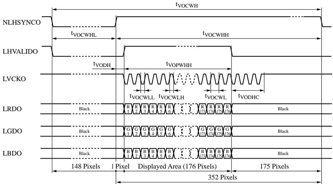
Note) When H\_POS = 1, pixel 0 and pixels 177 to 351 will be filled with black in the LCD RGB, and only pixels 1 to 176 will be output.
