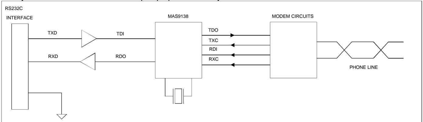
**◆ Synchronous serial interface with uP interface**
