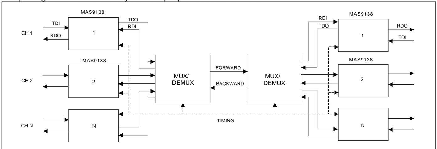
**◆ Synchronous modem with asynchronous interface**
