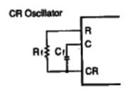
The values of R, and C, are typical values. The oscillation frequency varies with the mounting condition. Adjust oscillation frequency to the required value.
