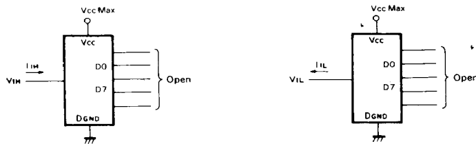
Test circuit of digital input current (CLK, MINV, LINV)
