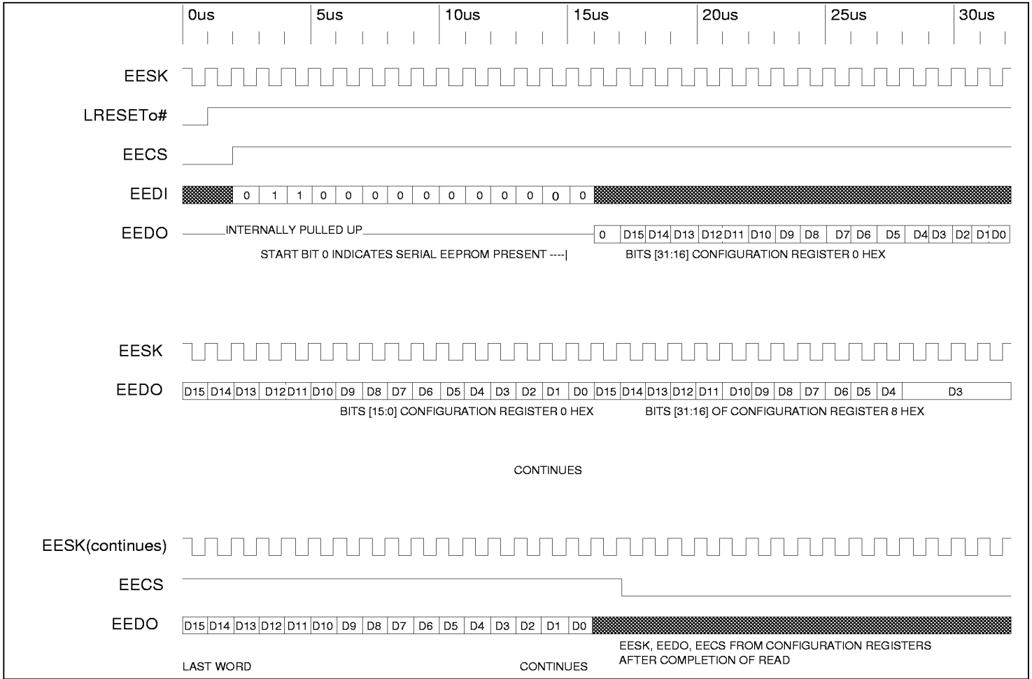
Timing Diagram 2-2. Initialization from Serial EEPROM (4K)
