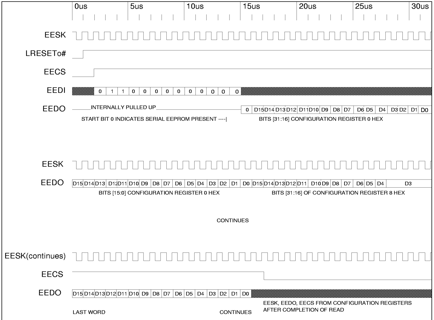
Timing Diagram 3-26. Initialization from Serial EEPROM (2K)
