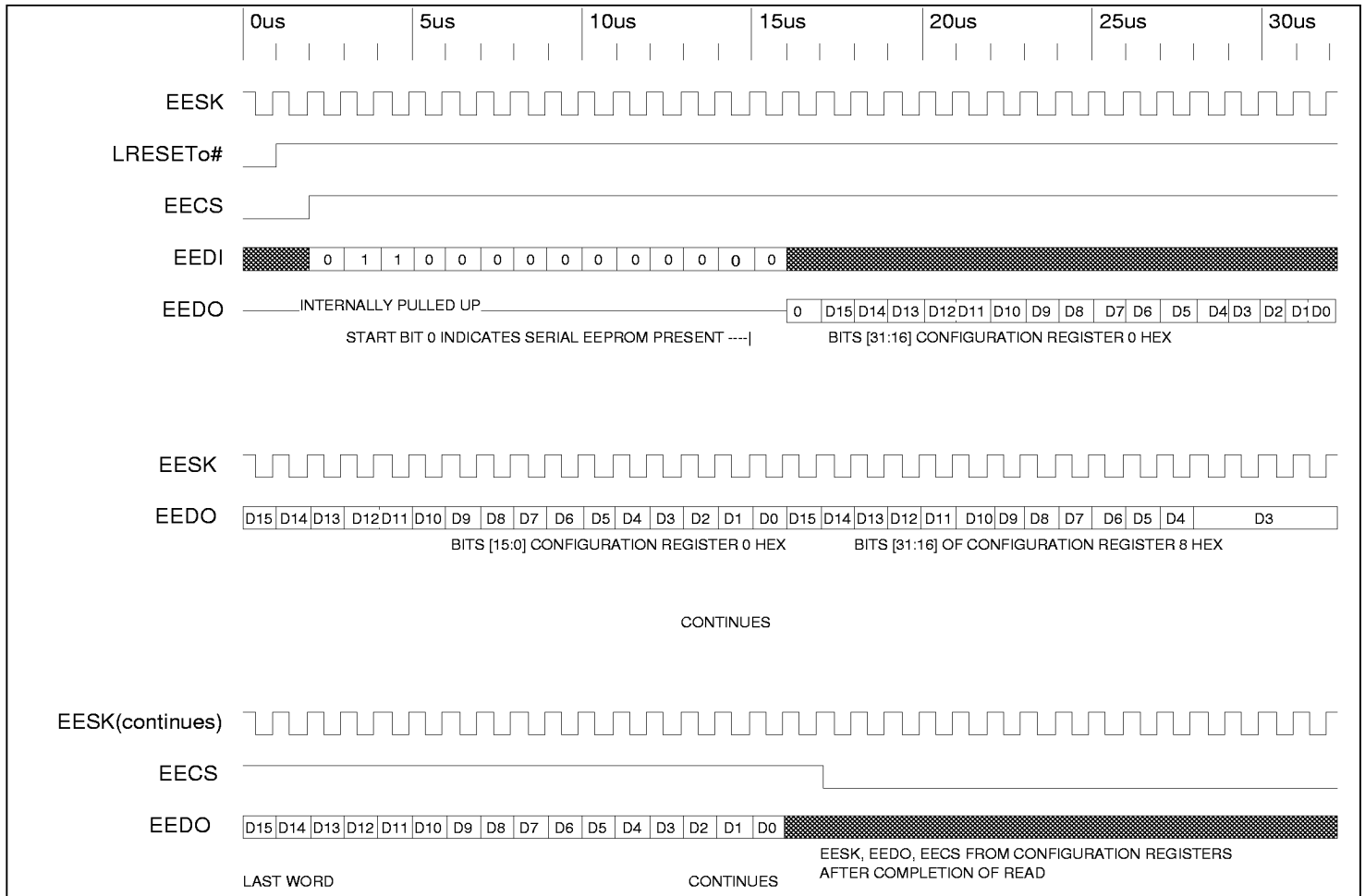
Timing Diagram 3-27. Initialization from Serial EEPROM (4K)
