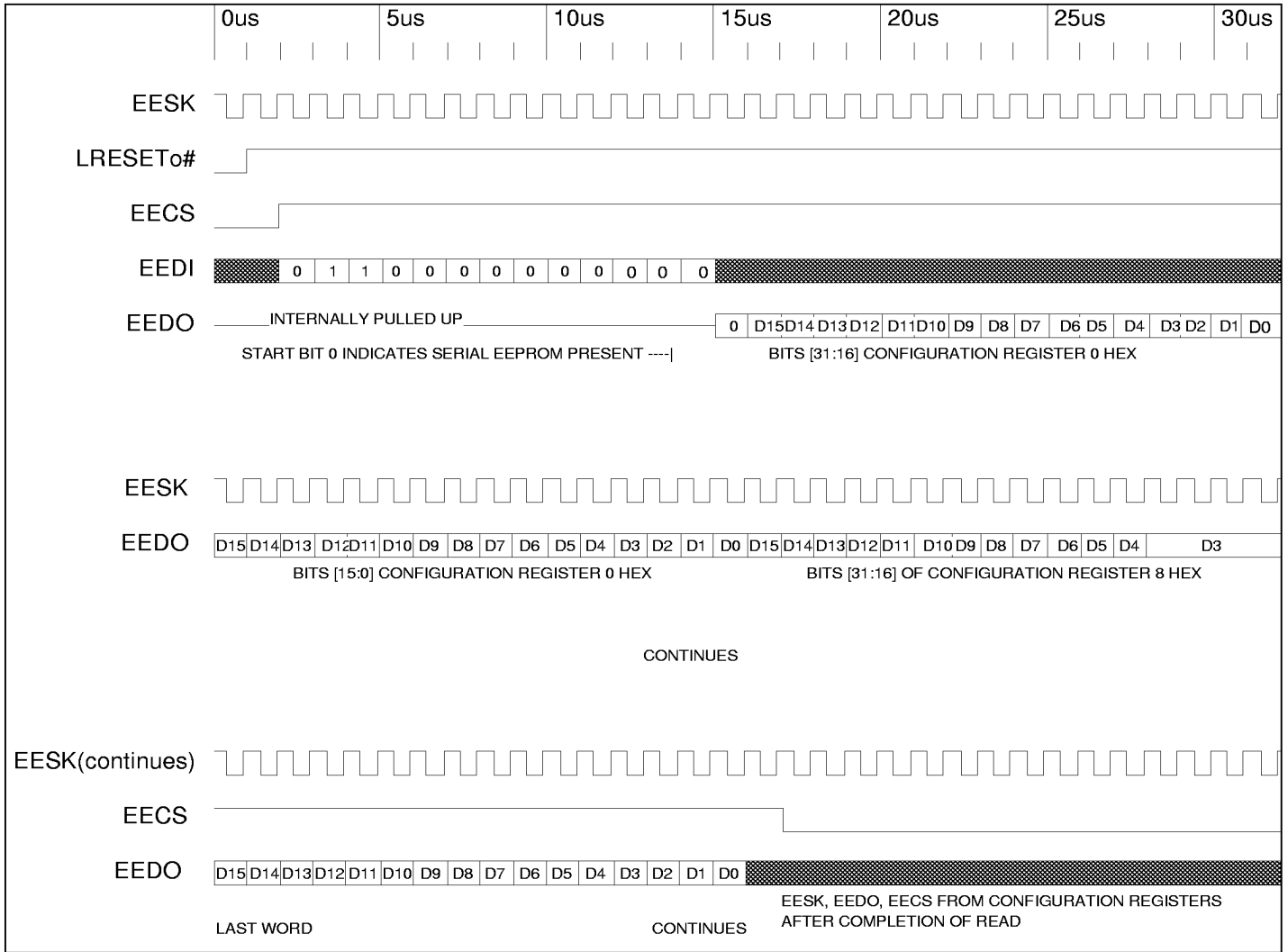
Timing Diagram 4-1. Initialization from Serial EEPROM (2K)
