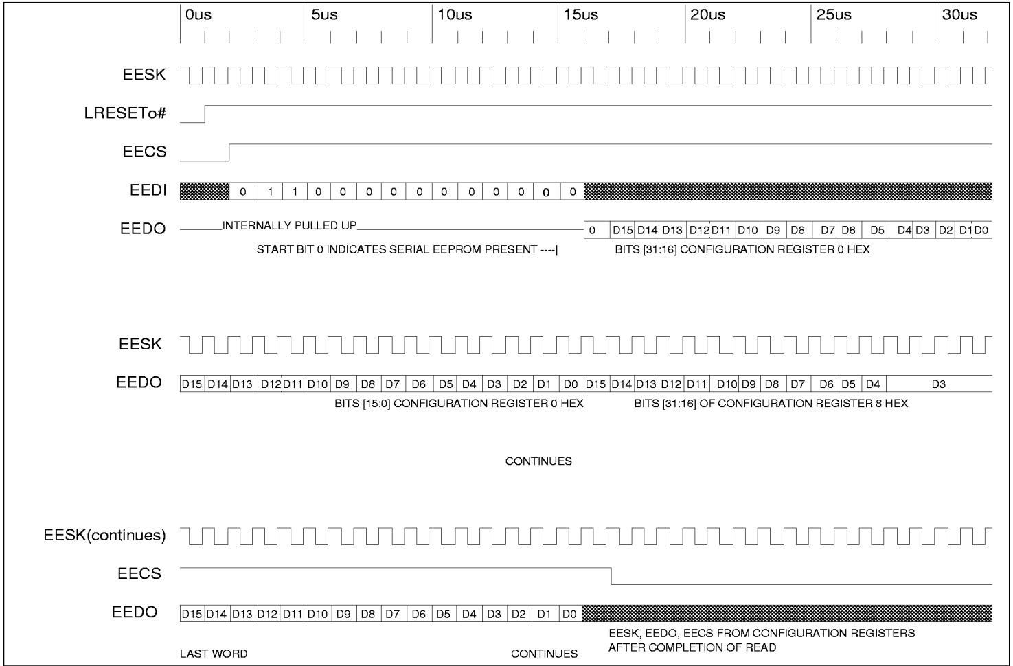
Timing Diagram 5-18. Initialization from Serial EEPROM (4K)
