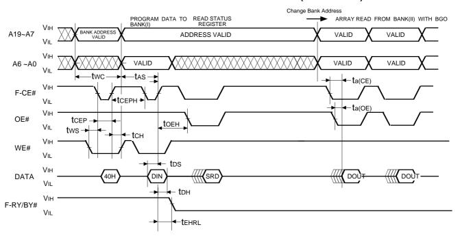
16,777,216-BIT (1,048,576 -WORD BY 16-BIT) CMOS 3.3V-ONLY FLASH MEMORY & 4,194,304-BIT (524,288-WORD BY 8-BIT) CMOS SRAM Stacked-MCP (Multi Chip Package)
