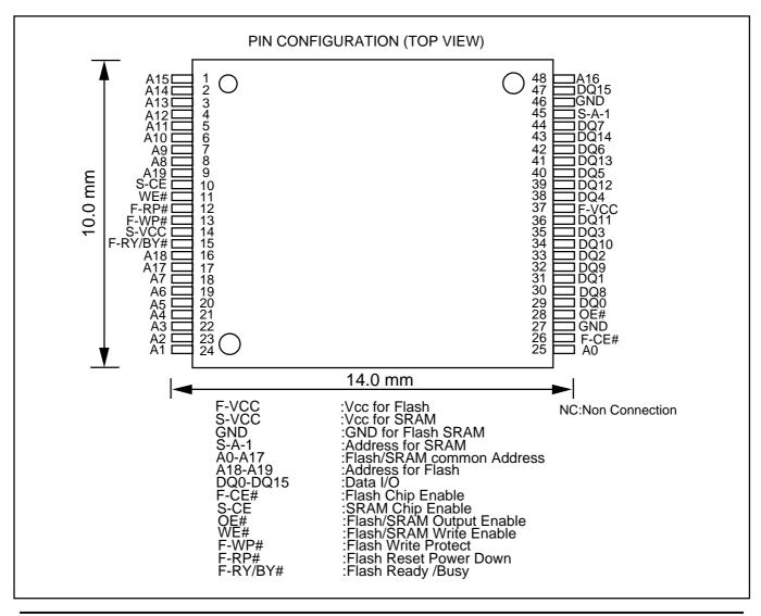
16,777,216-BIT (1,048,576 -WORD BY 16-BIT) CMOS 3.3V-ONLY FLASH MEMORY & 4,194,304-BIT (524,288-WORD BY 8-BIT) CMOS SRAM Stacked-MCP (Multi Chip Package)
