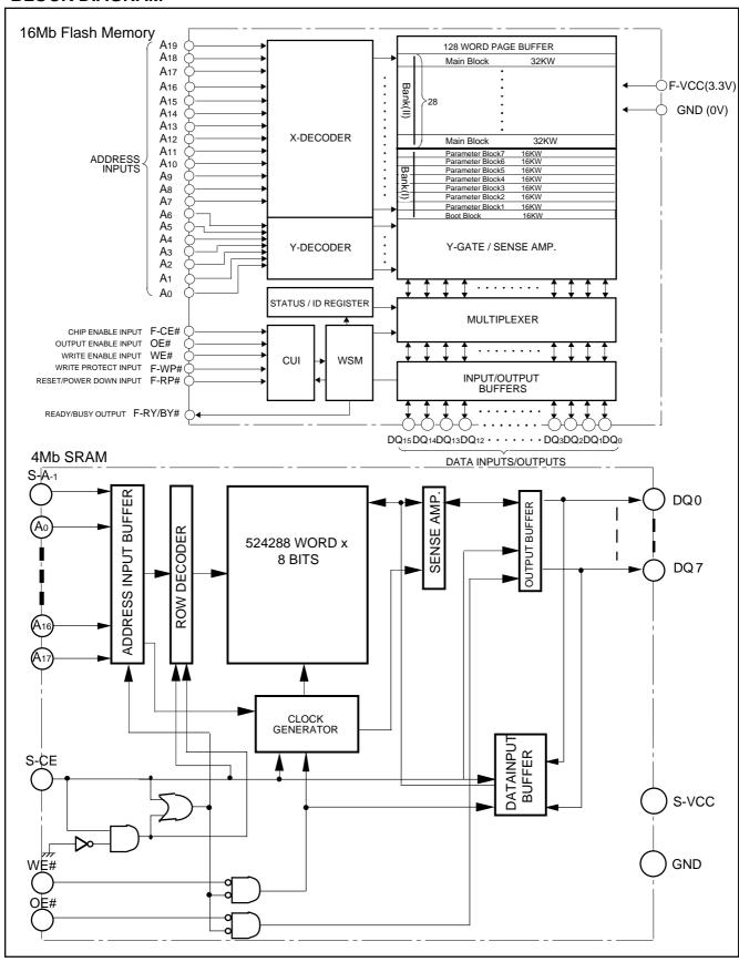
M6MGB/T162S4BVP 16,777,216-BIT (1,048,576 -WORD BY 16-BIT) CMOS 3.3V-ONLY FLASH MEMORY & 4,194,304-BIT (524,288-WORD BY 8-BIT) CMOS SRAM Stacked-MCP (Multi Chip Package)
