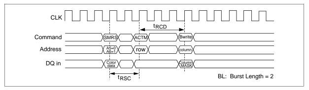
Block Write Example with Write Per Bit
