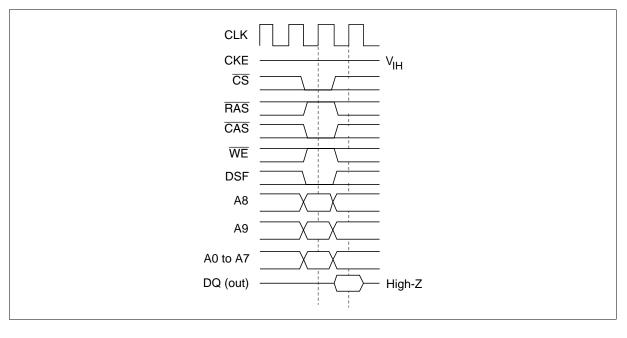
Column address and write command: For a row of one of two banks activated by ACTV or ACTVM, at
