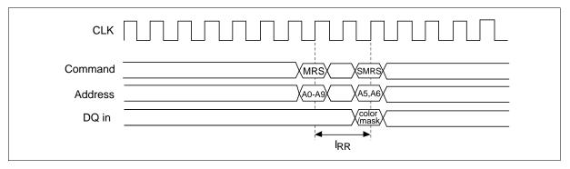
**Special Mode Register Set to Block Write/Write Interval:** The minimum interval between a special mode register set and a block write/write is t<sub>SBW</sub>.
