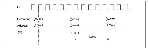
**Block write with auto-precharge:** In this operation, since precharge is automatically performed after completion of a block write operation, so no need to execute precharge command. The following command must be a bank active command (ACTV, ACTVM). In addition, an interval of  $l_{APBW}$  is required between the last valid data input and the following command.
