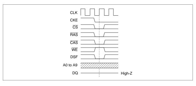
No operation command (NOP): At the CLK rising edge, by setting  $\overline{CS}$ ; LOW, WE,  $\overline{RAS}$ ,  $\overline{CAS}$ ; HIGH, [State transition] No transition
