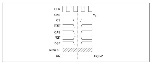
Self refresh command (REF): If both banks are in idle state, at the CLK rising edge, by setting CS, RAS, CAS, DSF; LOW, WE; HIGH, and if CKE's falling edge is detected, the HM5283206 starts self-refresh operation. Self-refresh operation is kept while CKE is LOW. [State transition] Idle — (Self refresh command) -> Self refresh mode
