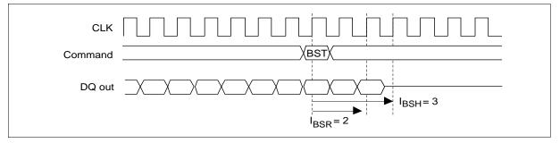
**Burst stop command at burst write:** For full page burst write cycle, when a burst stop command is issued, the write data at that cycle and the following write data input are ignored. The BST command is legitimate only in case full page burst mode, and is illegal for burst length 1, 2, 4 or 8.
