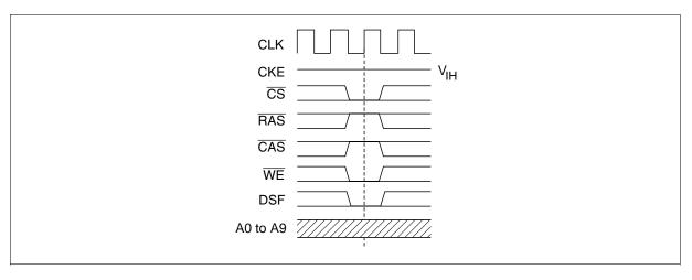
Auto refresh command (REF): If both banks are in idle state, at the CLK rising edge, by setting CS, RAS, CAS, DSF; LOW, WE; HIGH, the HM5283206 starts auto-refresh (CBR type) operation. Refresh address is internaly generated.
