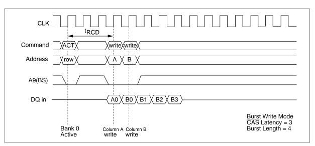
2. Operation for a column in other row of the same bank: It is necessary to execute a precharge command and a bank active command before executing the following write command.
