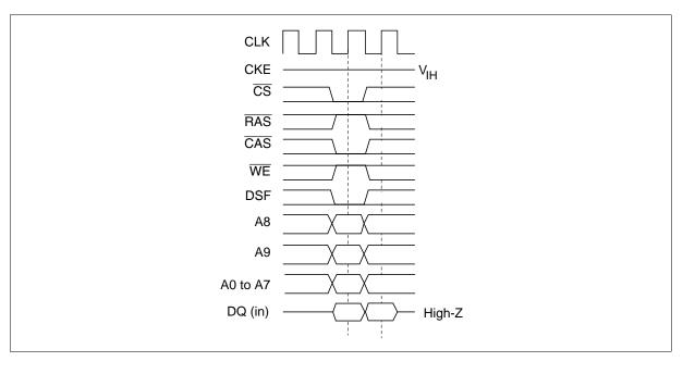
**Burst stop command (BST):** At the CLK rising edge, by setting  $\overline{CS}$ ,  $\overline{WE}$ , DSF: LOW, RAS,  $\overline{CAS}$ ; HIGH, full page burst (BL = 256) read/write is interupted. If BL is set to 1, 2, 4, 8, to try to execute this command is illegal. [State transition] Row active — (Burst stop command) -> Row active
