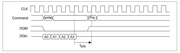
Block Write Command to Precharge Command Interval: The minimum interval between block write command and the following precharge command is  $t_{BWR}$ .
