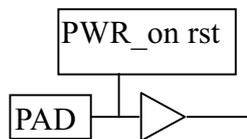
(7) Pin22~25 , Pin27~30(GPIO0~7) : Bi-directional I/O buffer with programmable pull-up/down resistor
