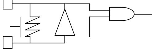
(5) Pin15, 16, 18(ECS , EDI , ESCK) , Pin43(SEN) , Pin46(AECNT) , Pin50(MCLK) : Output buffer PAD
