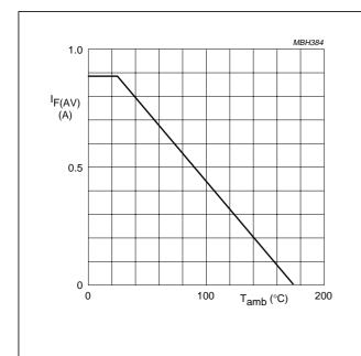
Fig.2 Maximum average forward current as a function of ambient temperature.
