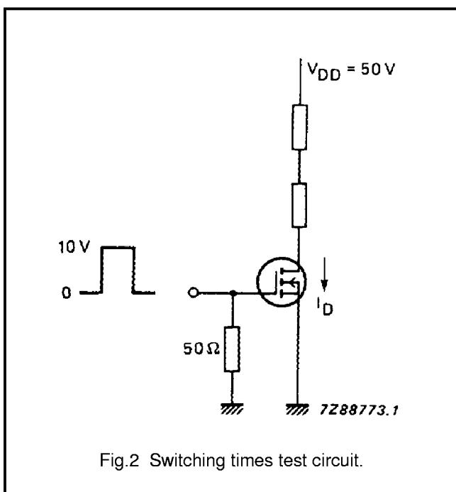
Fig.2 Switching times test circuit.
