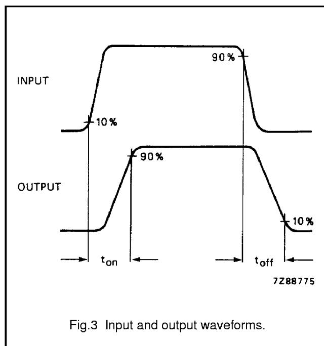
Fig.3 Input and output waveforms.
