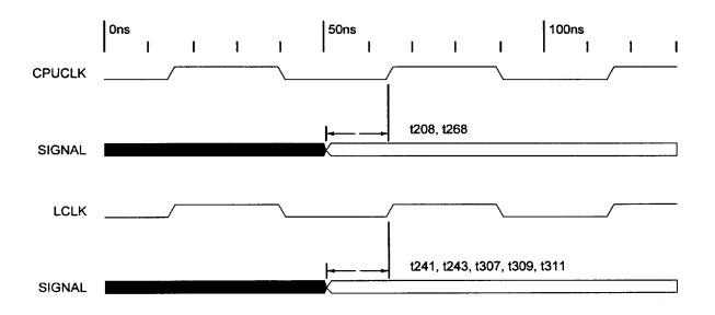
Figure 6-3 Output Delay Timing Waveform
