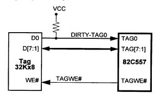
Figure 4-19 32Kx8 and 32Kx8 Combined Tag/Dirty RAM Implementation (Separate Devices)
