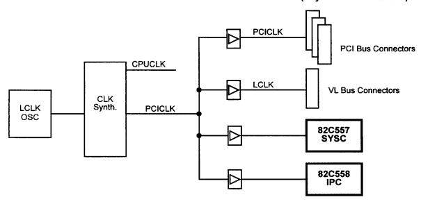
Figure 4-3 Clock Distribution Method for VL Bus and PCI Connectors (Sync. PCI and VL Bus)
