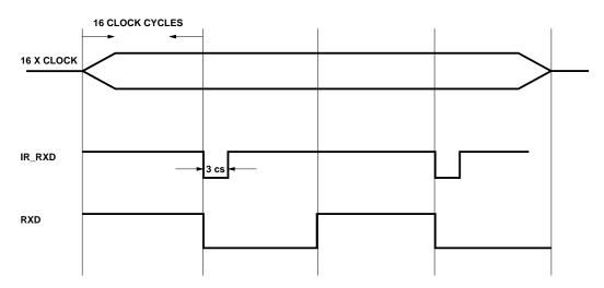
A high to low transition of the IR\_RXD line from the HSDL-1000 signifies a 3/16th pulse. This pulse is stretched to accommodate 1 bit time (16 clock cycles). Every pulse that is received is
