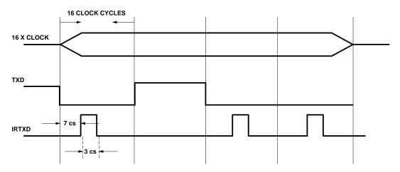
The encoder sends a pulse for every space or "0" that is sent on the TXD line. On a high to low transition of the TXD line, the generation of the pulse is delayed
