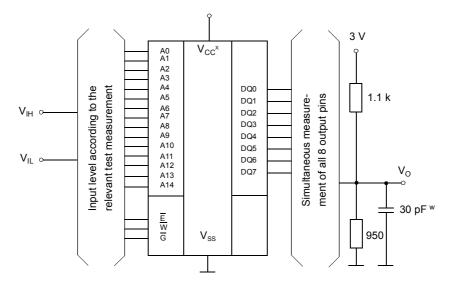
w: In measurement of  $t_{dis}$ -times and  $t_{en}$ -times the capacitance is 5 pF.
