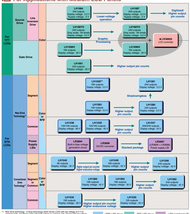
New drive technology: A drive technology which drives LCDs with low voltage of 5 V on segment side, and drives LCDs with high voltage on common side. Driving with low voltage on segment side enables LCDs to reduce power consumption and shadowing. Conventional drive technology: A drive technology which drives LCDs with high voltage on both segment and common sides.
