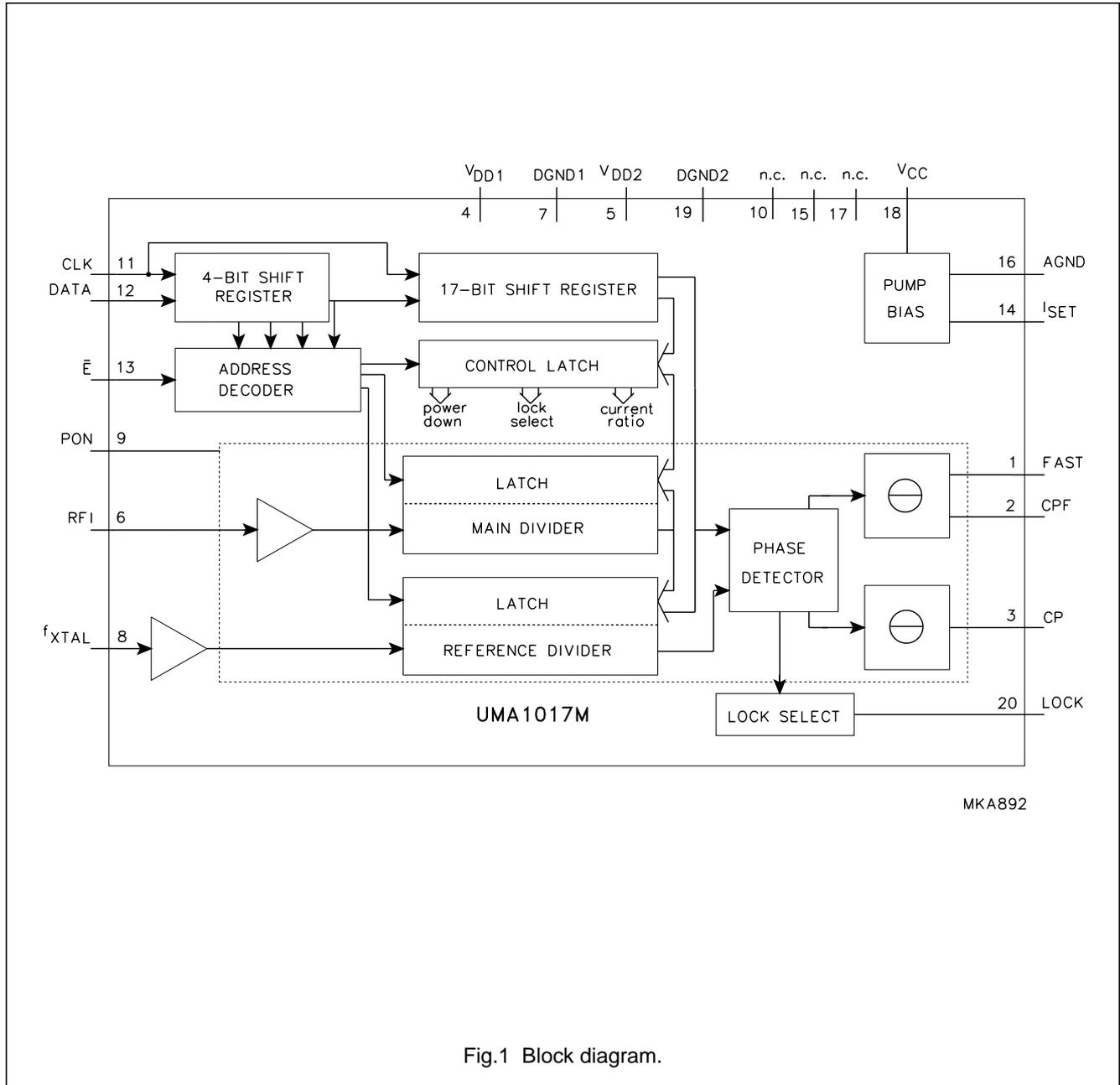
Fig.1 Block diagram.
