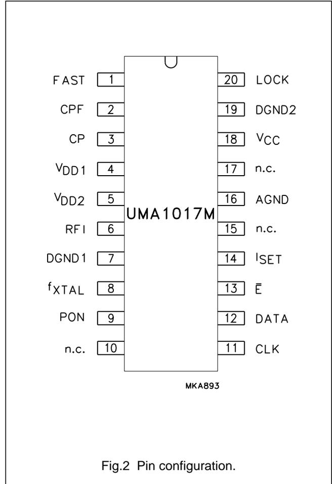
Fig.2 Pin configuration.
