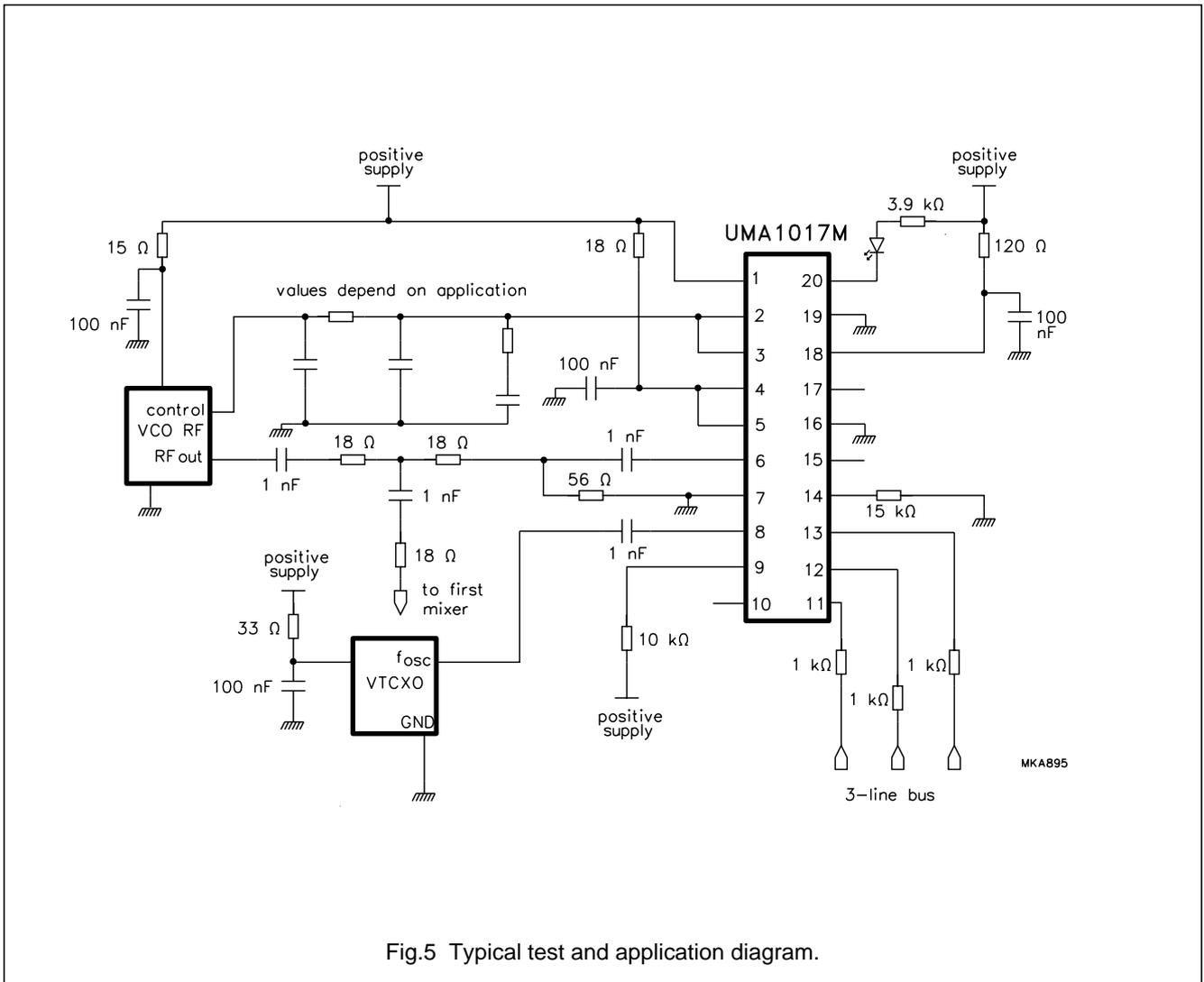
Fig.5 Typical test and application diagram.
