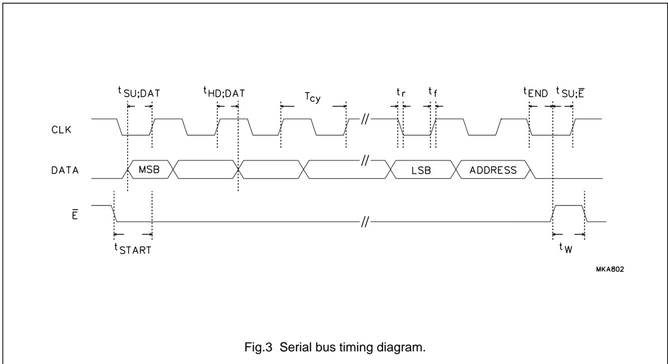
Fig.3 Serial bus timing diagram.
