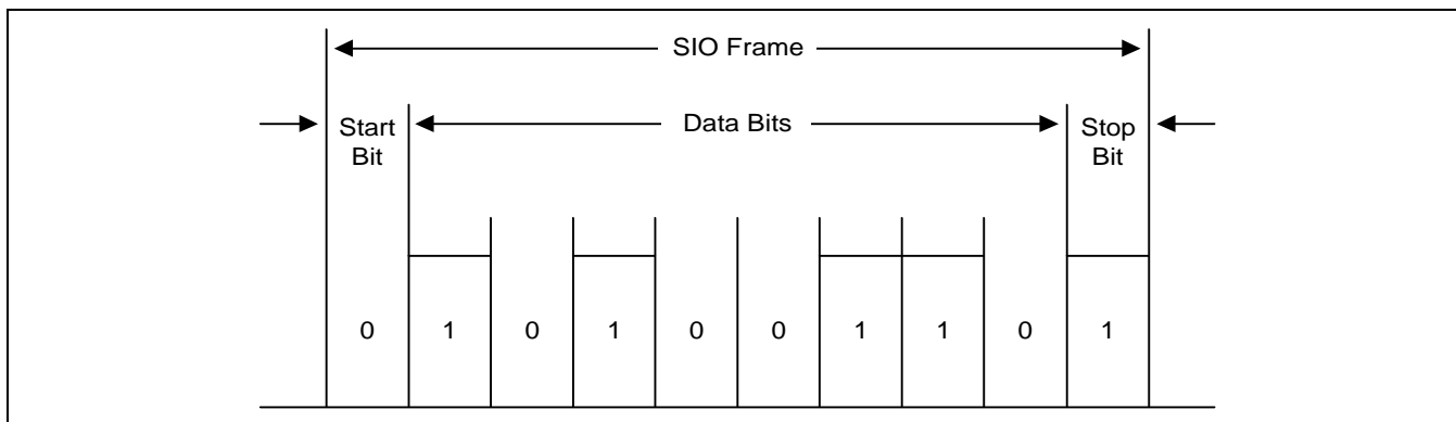
Figure 11-4. Serial I/O Frame Timing Diagram (Normal UART)
